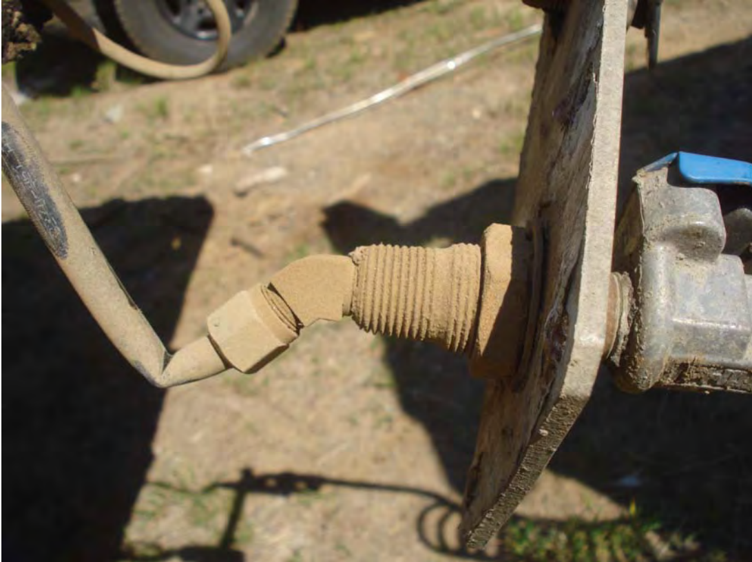
Bulk head removed showing kinked air line on service side
