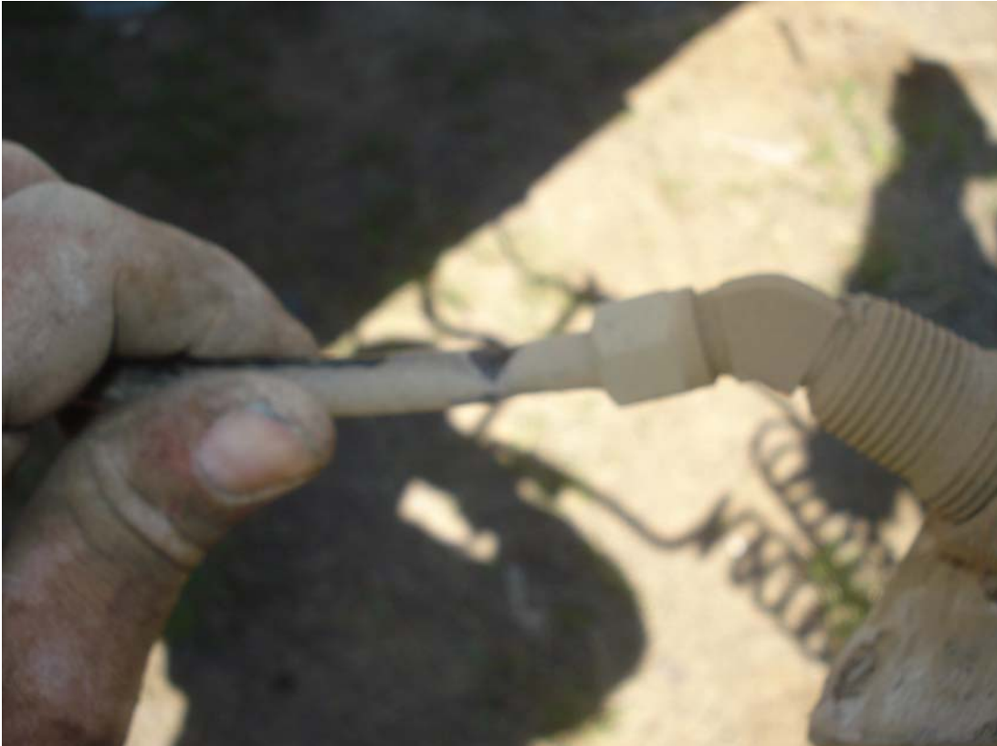
Same air line as above straightened out indicating pre-existing condition
