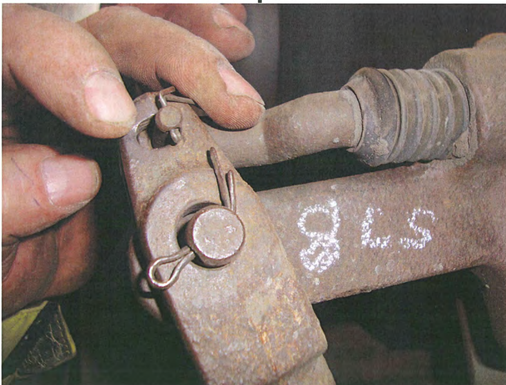
Photo # 12 – axle #8 left push rod, worn clevis and pins
