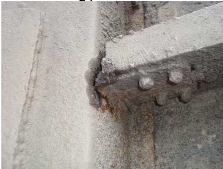
Photo # 10 – Crack in cross member at body mounting point of trailer #2
