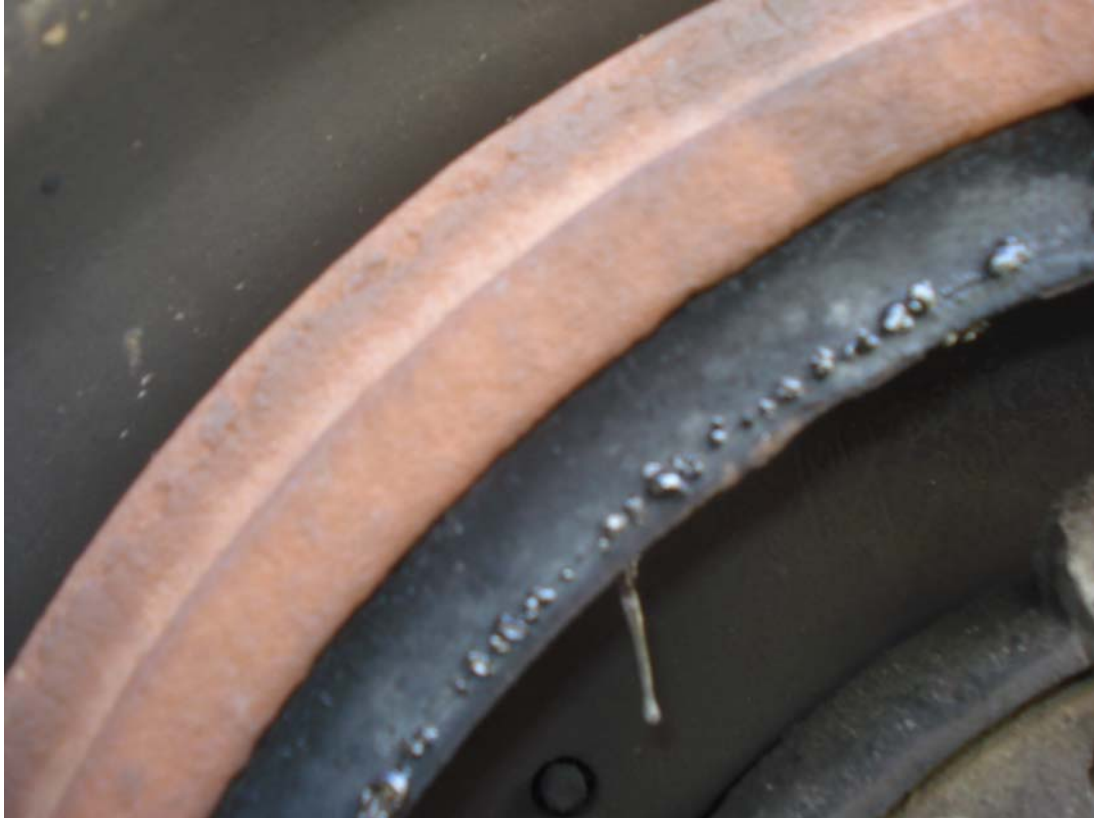
Axle 5 left showing drum discoloration and bonding material melted
