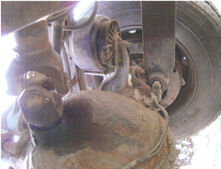
Photo # 14 – axle #3 right broken air bag pedestal
