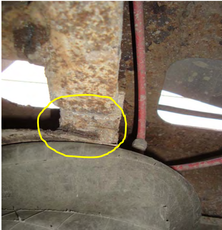
Photo # 9 – Cracks in cross member above axle #4 on trailer #1
