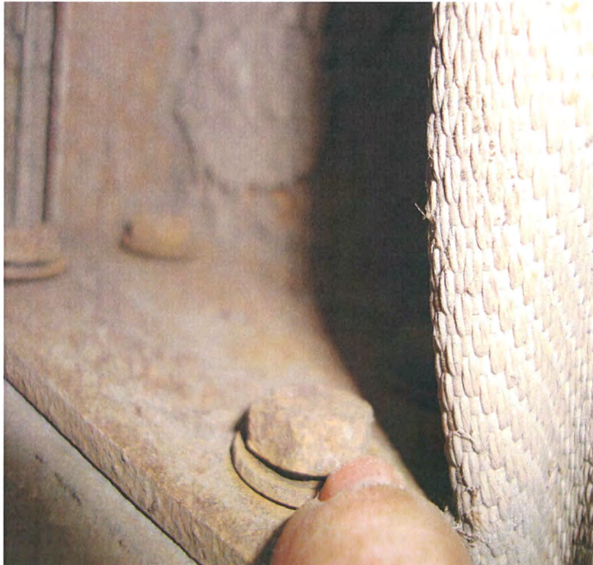
Photo # 16 – trailer #2 –loose frame bolts
