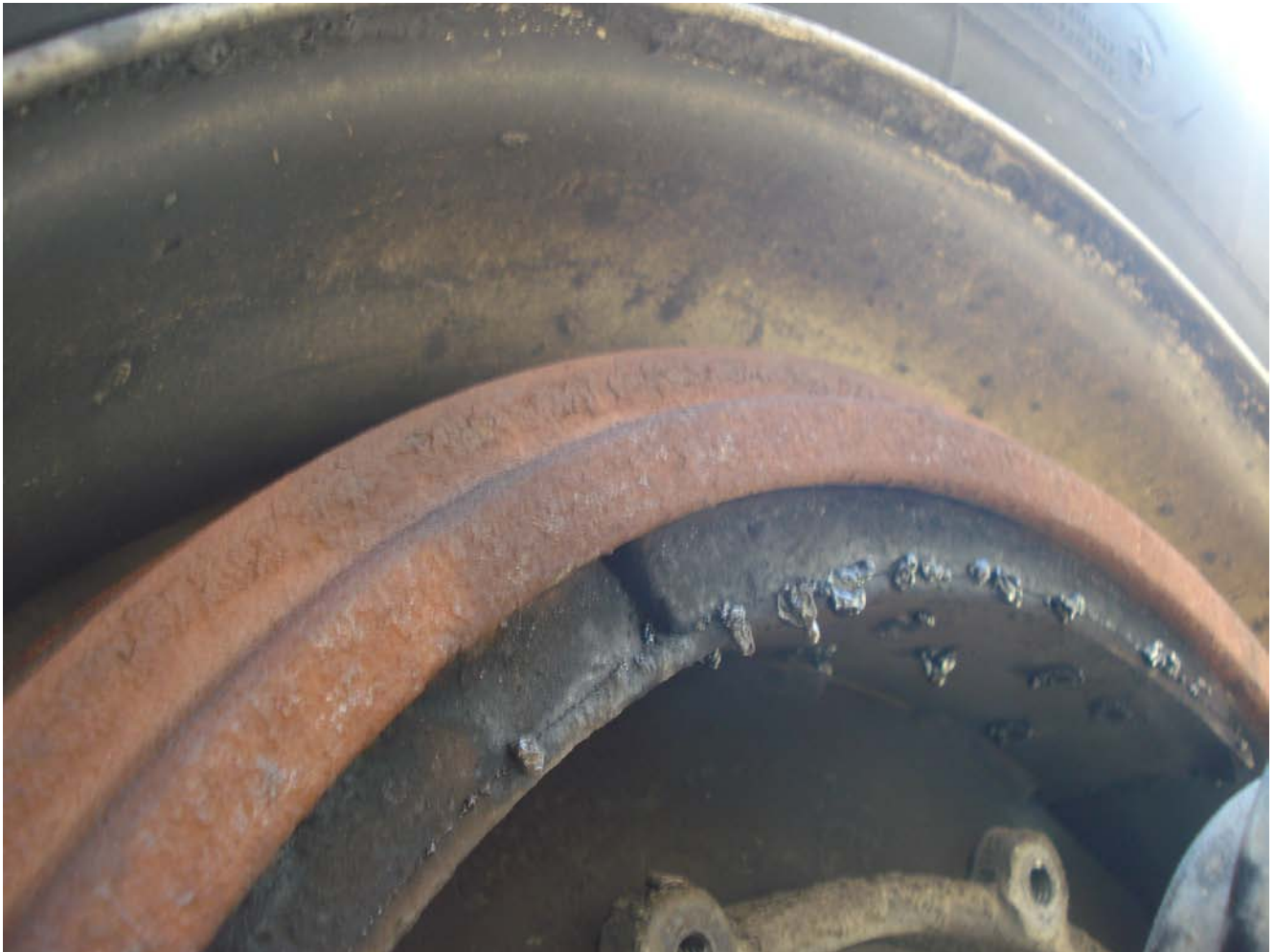
Axle 2 left showing drum discoloration and bonding material melted
