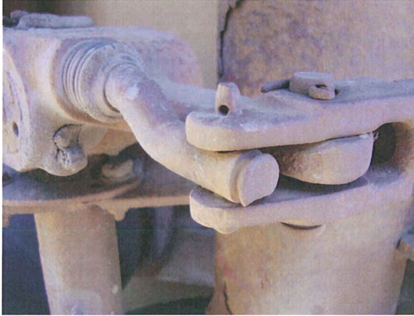
Photo # 14 – axle #3 right broken air bag pedestal
