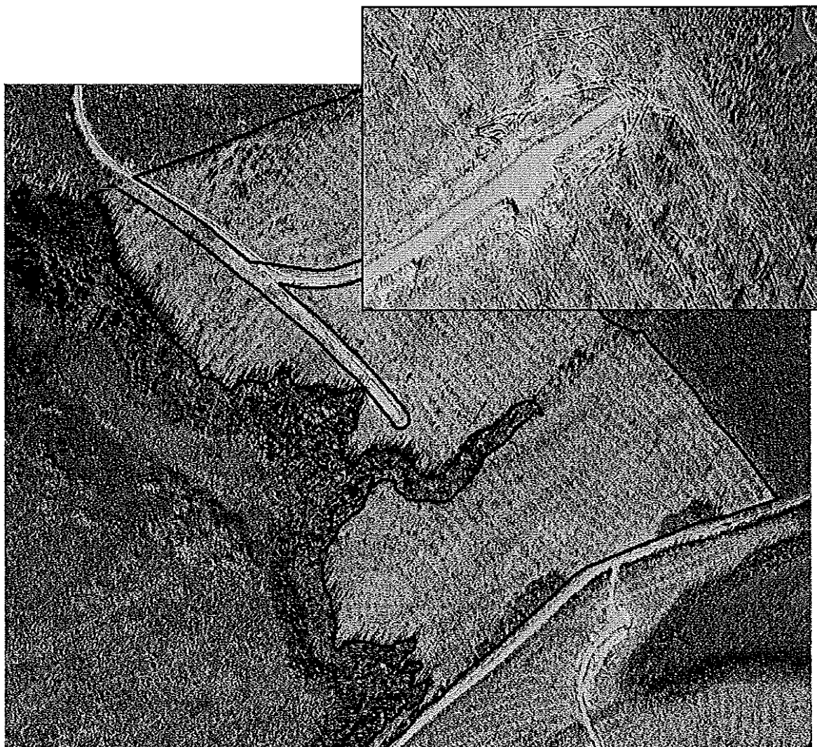
Figure 2. Aerial Photography of block CAR464 in 2010 (1 year post logging, 15 cm pixel size resolution). Insert shows the extent of ruts and ponded water in northwest area.
