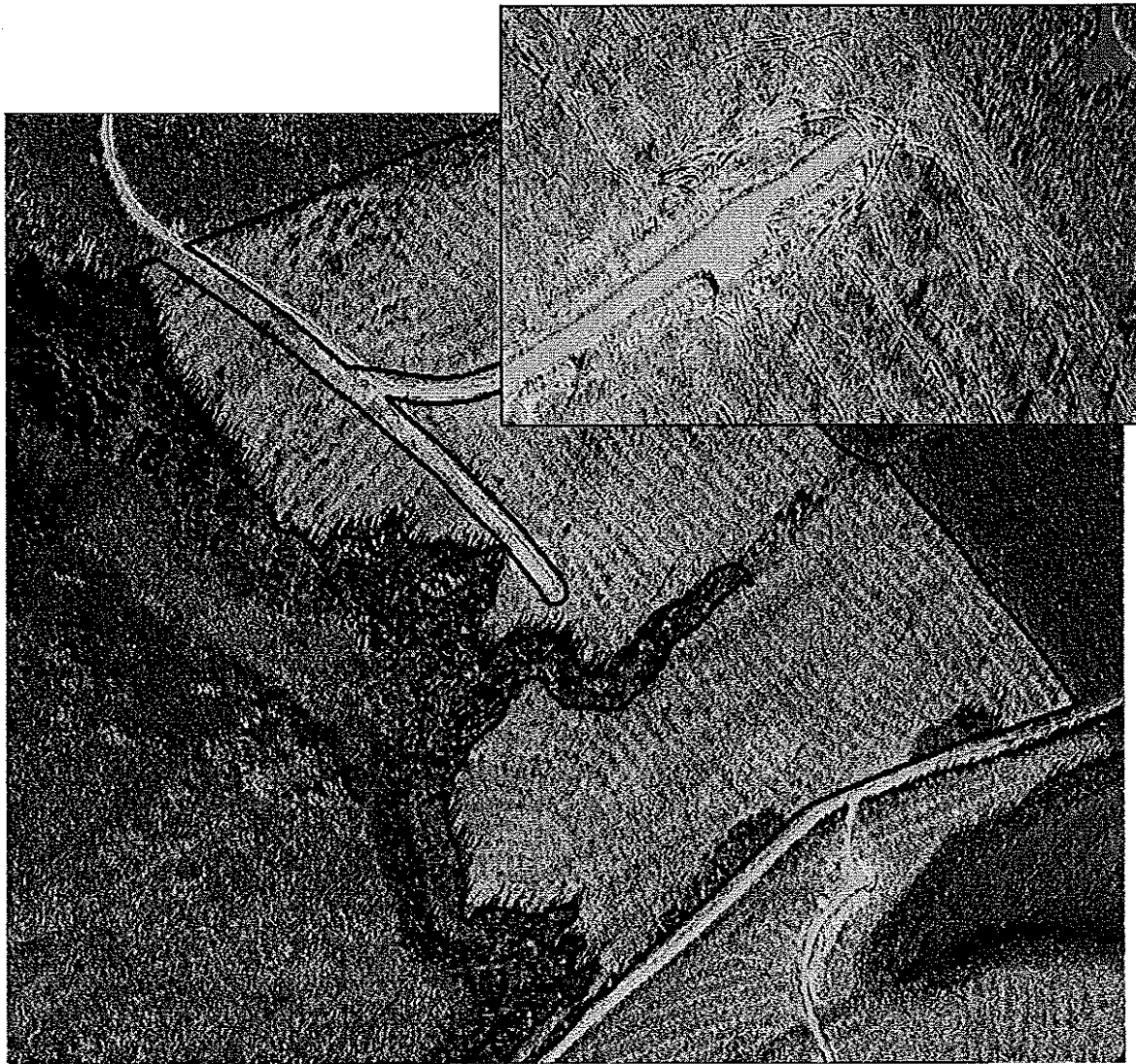
Figure 1. Aerial Photography of block CAR464 in 2010 (1 year post logging, 15 cm pixel size resolution). Insert shows the extent of ruts and ponded water in northwest area.
