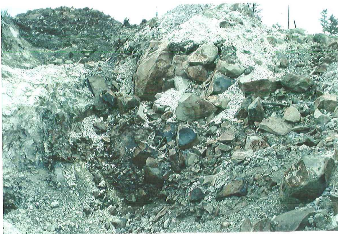
Excavator trench - exposed basalt cap rock ,Beppe Pit south.
