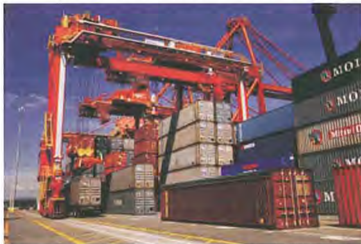
A gantry crane loads a shipping container onto a truck at Port Metro Vancouver's Centerm Terminal.
