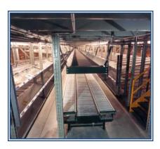
4) ASRS: Automated Storage and Retrieval System is used to minimize putaway and replenishment activities and reduce the building footprint by going vertical. ASRS with integrated pick tunnels is used, where fast moving SKUs are slotted at the bottom level of ASRS and replenished automatically. Other SKUs are also stored in the ASRS system, but once retrieved they need to be manually replenished into the pick locations that are outside of ASRS system.
