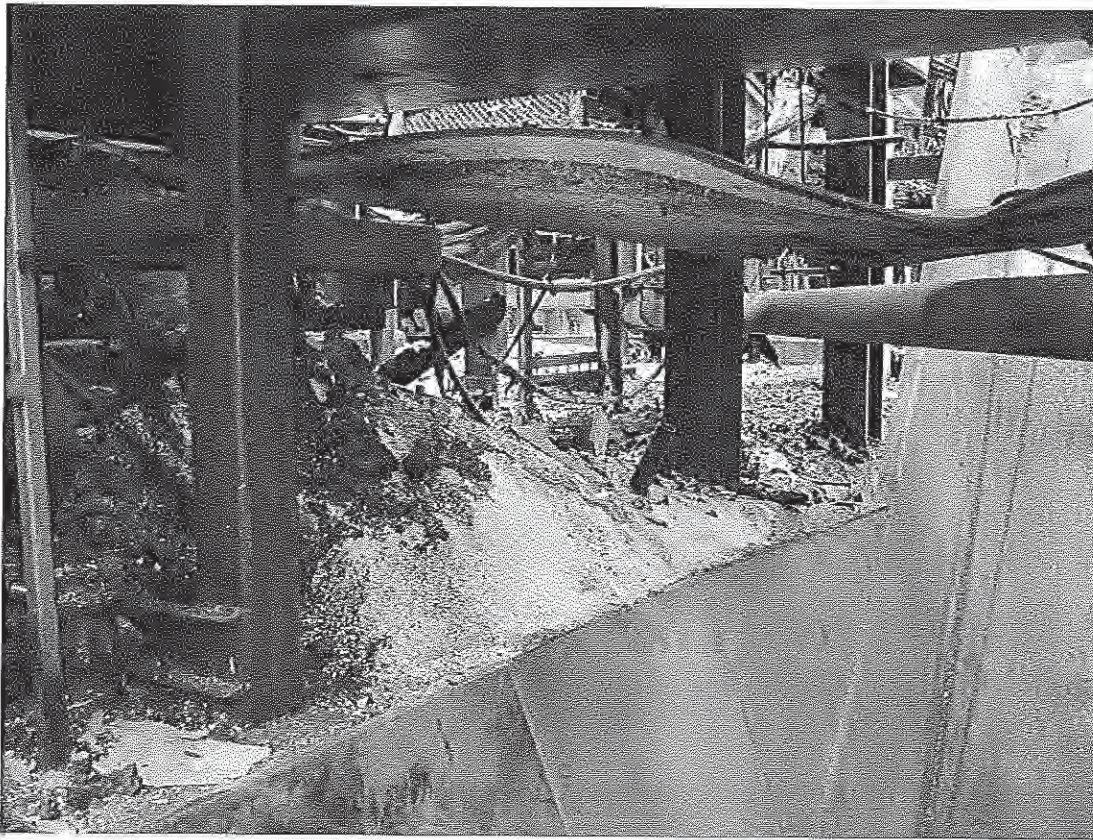
Figure 11: Excessive wood waste build-up was found behind the motor assembly.
