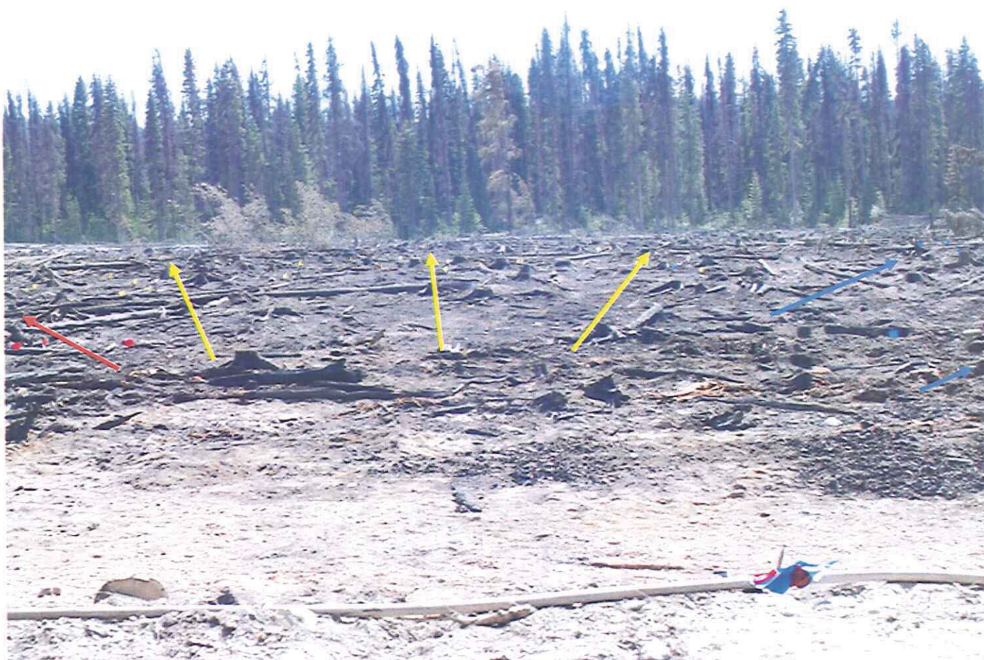
DSC_0010: Photo taken from Location 003, bearing 205°, from the road. Investigators were able to follow advancing, lateral and backing fire vector indicators to the Area of Origin, which is where the processor had been processing logs prior to the start of the fire. Note the intense burn in the Area of Origin.
