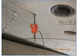
RM-3 is in near perfect orientation with the tunnel since the data were recorded from geophones connected to the ceiling very near the crown. Given that, the interpretation is judged to be more representative of conditions directly over the alignment minus a "blind zone" in near proximity to the tunnel.
