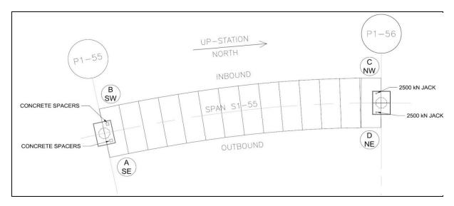
Span 1-55 is 42 metres in length, consisting of 14 precast concrete segments, with a total weight of 370 tonnes. The geometry of the beam is in a horizontal curve with a minimum radius of 162 metres at the approximate centre of beam. At pier 56 there is a maximum cross-fall of 6.5% combined with a longitudinal grade of 3.8%. At pier 55 the cross-fall is 4.5% and the longitudinal grade is less than 1.0%.
