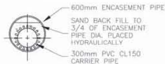
CARRIER PIPE AND ENCASEMENT PIPE INSTALLATION DETAIL
