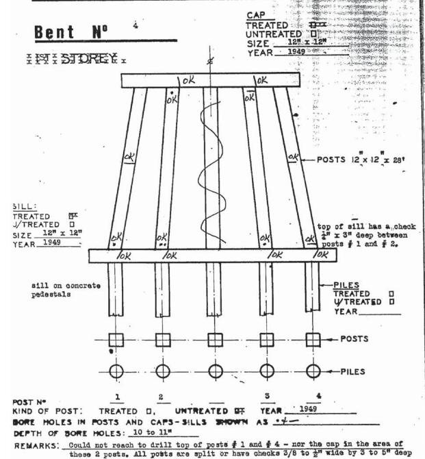
MOTE: Draw in major decay, internal and external, where found in each pile (or post). Show minimum and maximum shell thickness with all internal decay.
