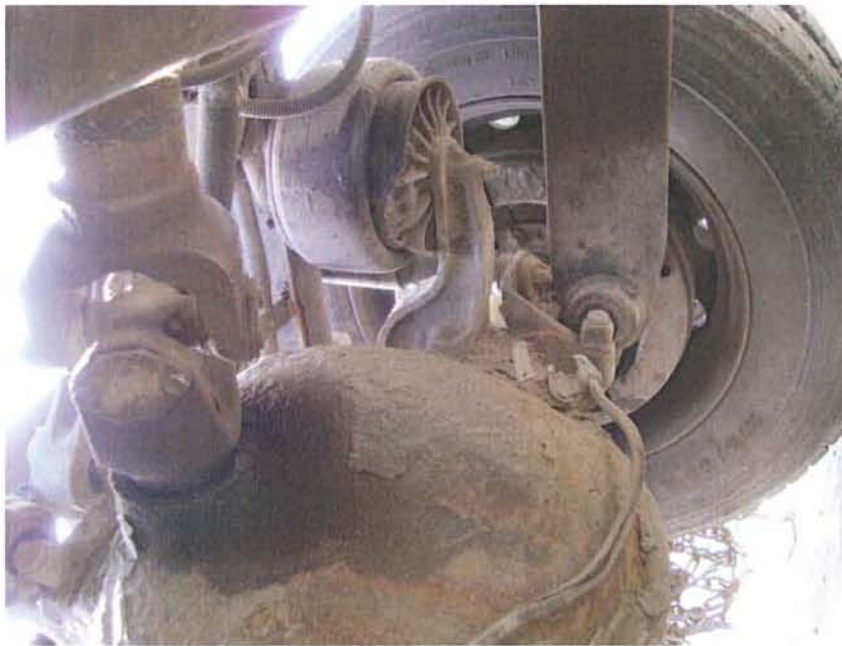
Photo # 14 – axle #3 right broken air bag pedestal
