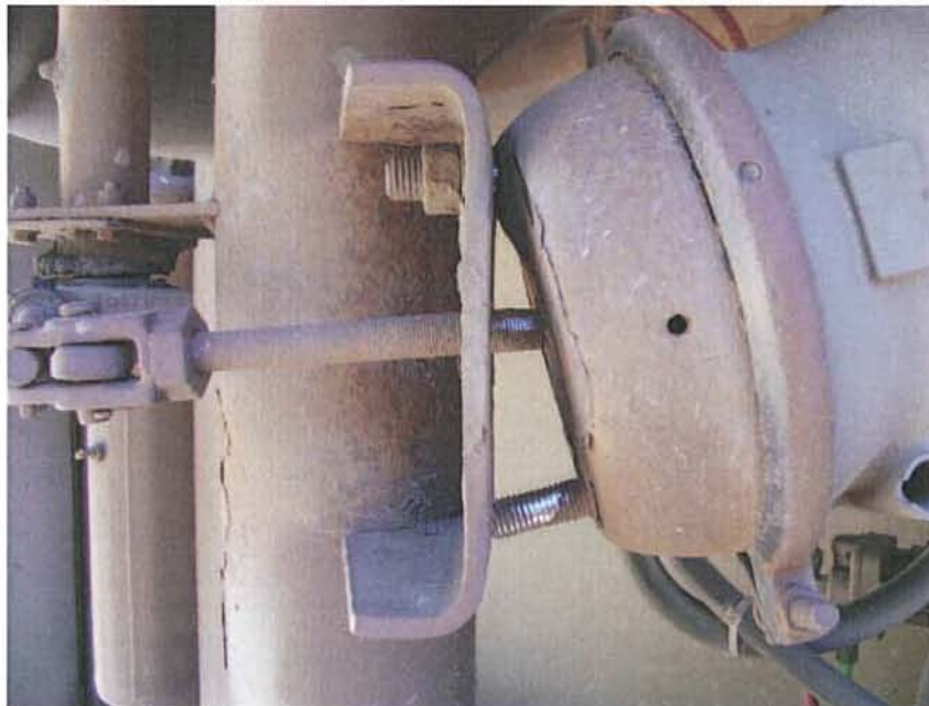
Photo # 10 – axle #9 loose brake chamber mount
