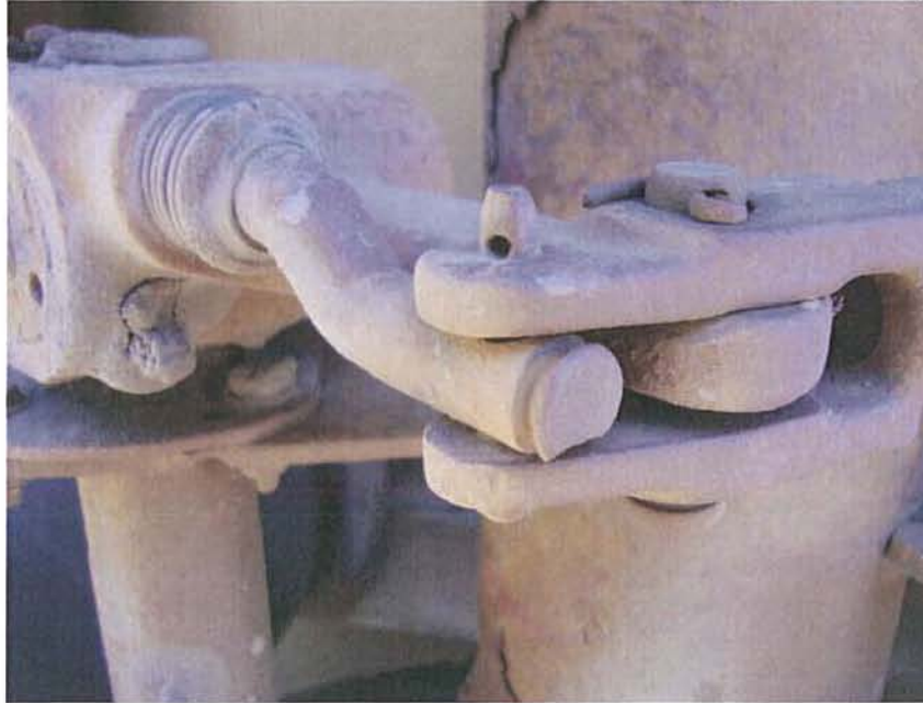
Photo # 14 – axle #3 right broken air bag pedestal
