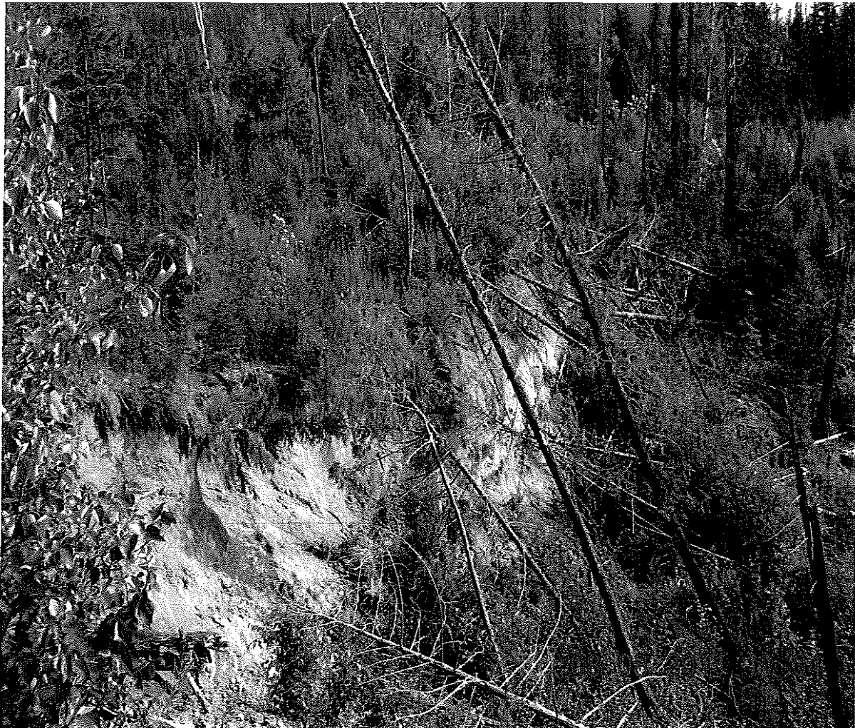
Photo #1 View of head scarp within block
