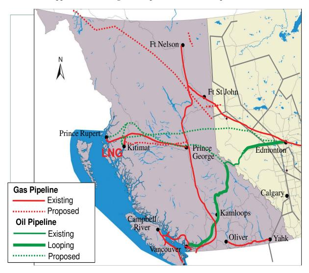
**Note:** The proposed Enbridge Northern Gateway pipelines project (GREEN dotted line) would move crude oil from Burderheim (60 km north of Edmonton) to tankers in a Kitimat terminal, as well as move condensate from tankers at Kitimat to Alberta.
