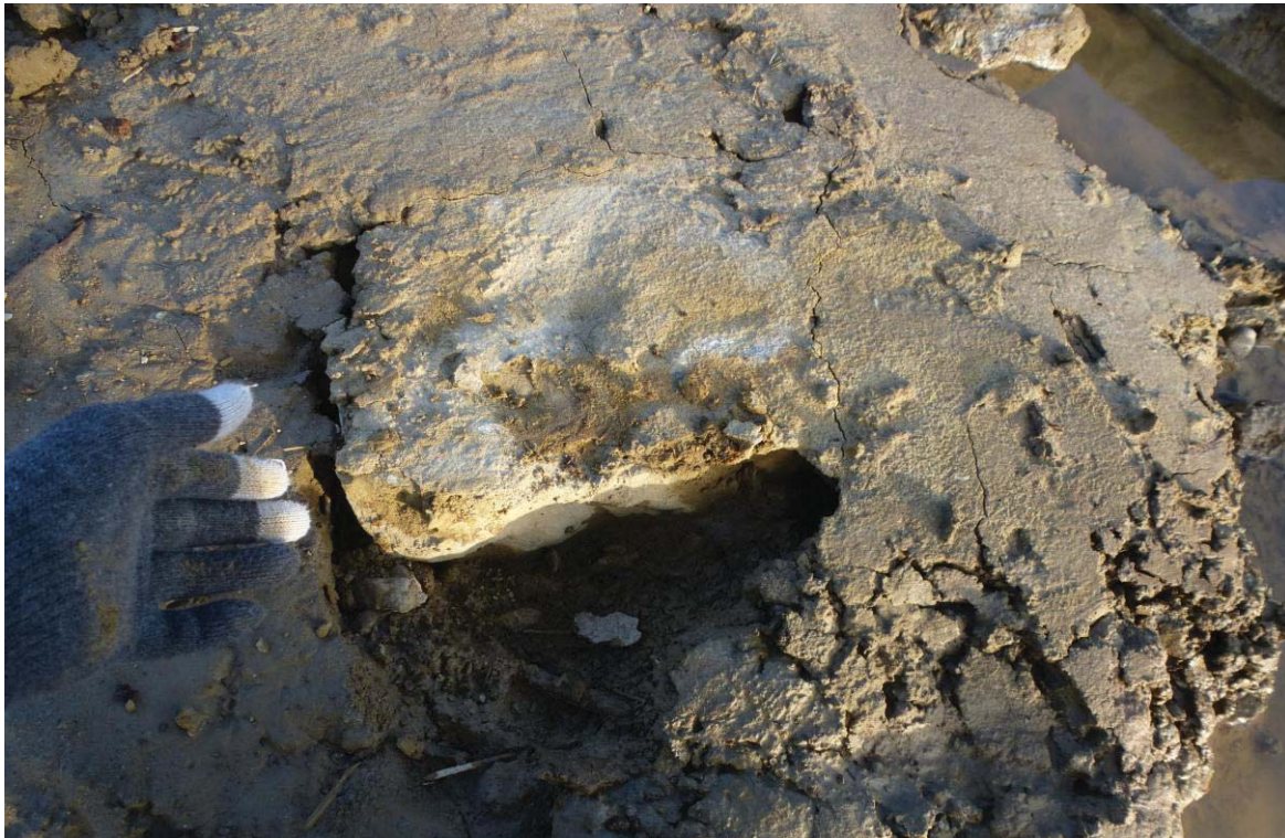
Figure 2: Eroding tailings at the banks of Hazeltine Creek, April 5 th 2015
