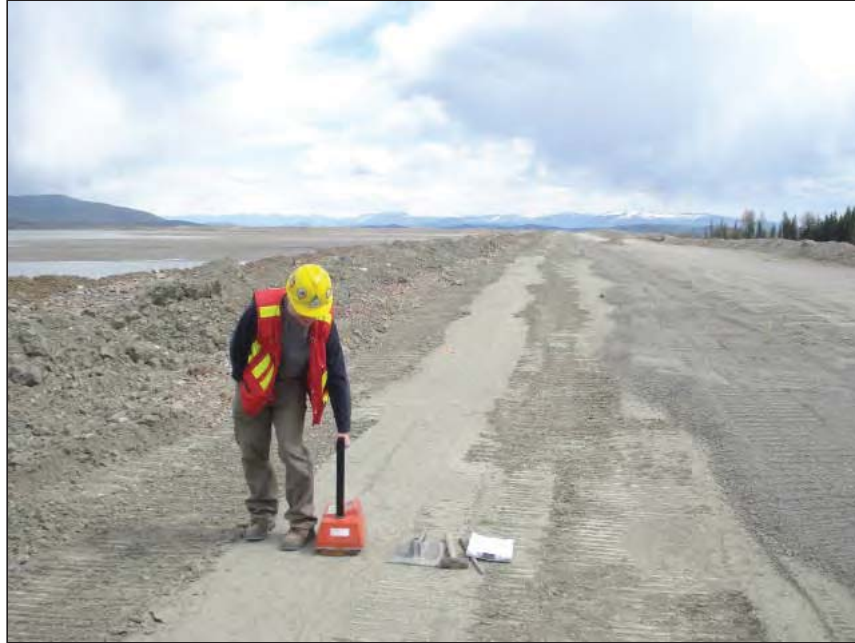
PHOTO 7 – Density testing of Zone S using a nuclear densometer on the South Embankment
