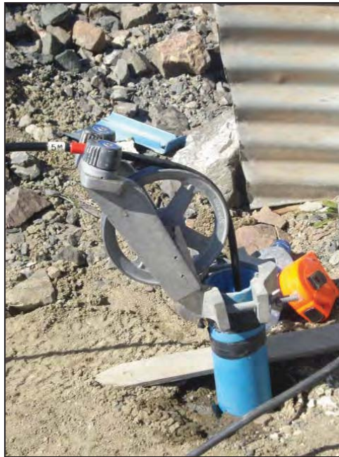
PHOTO 22 – Inclinometer measurements on the Main Embankment
