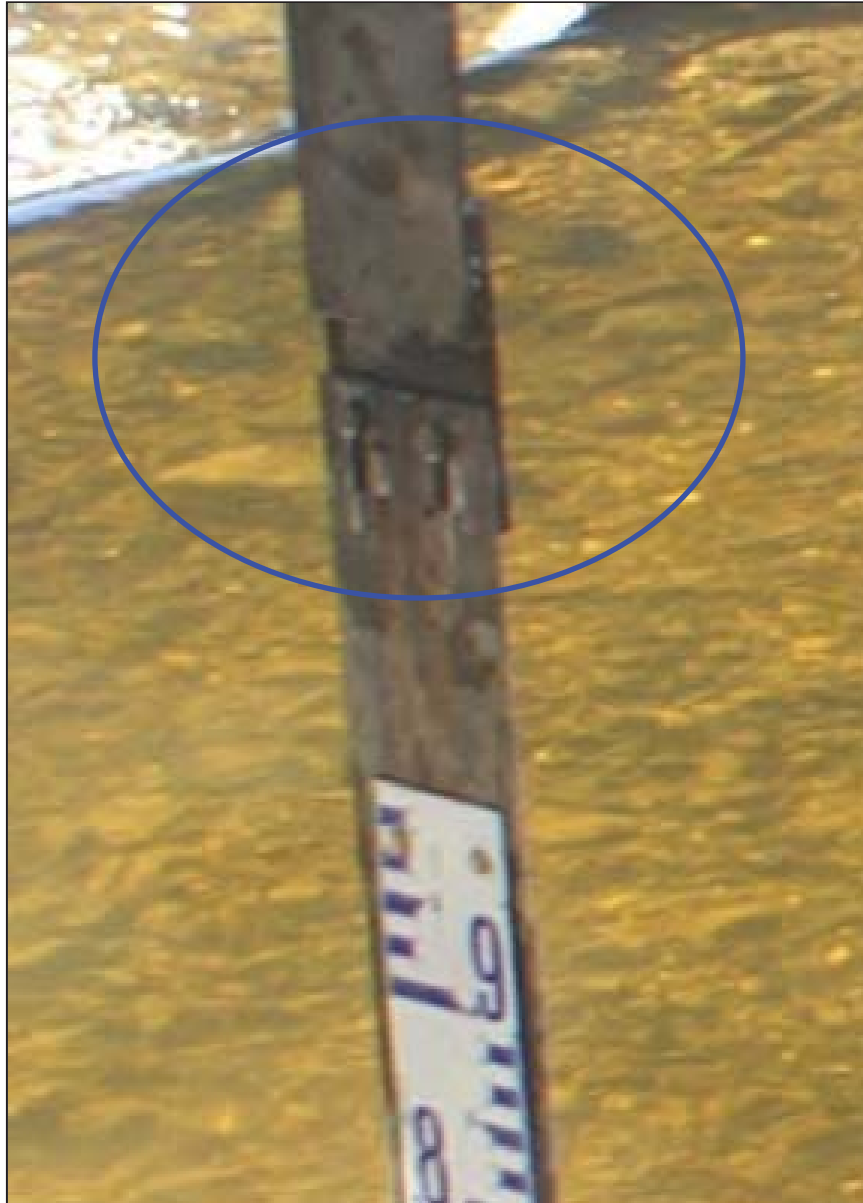
PHOTO 2 – Hazeltine Creek Gauging Station, new staff gauge installation showing removable lower portion
