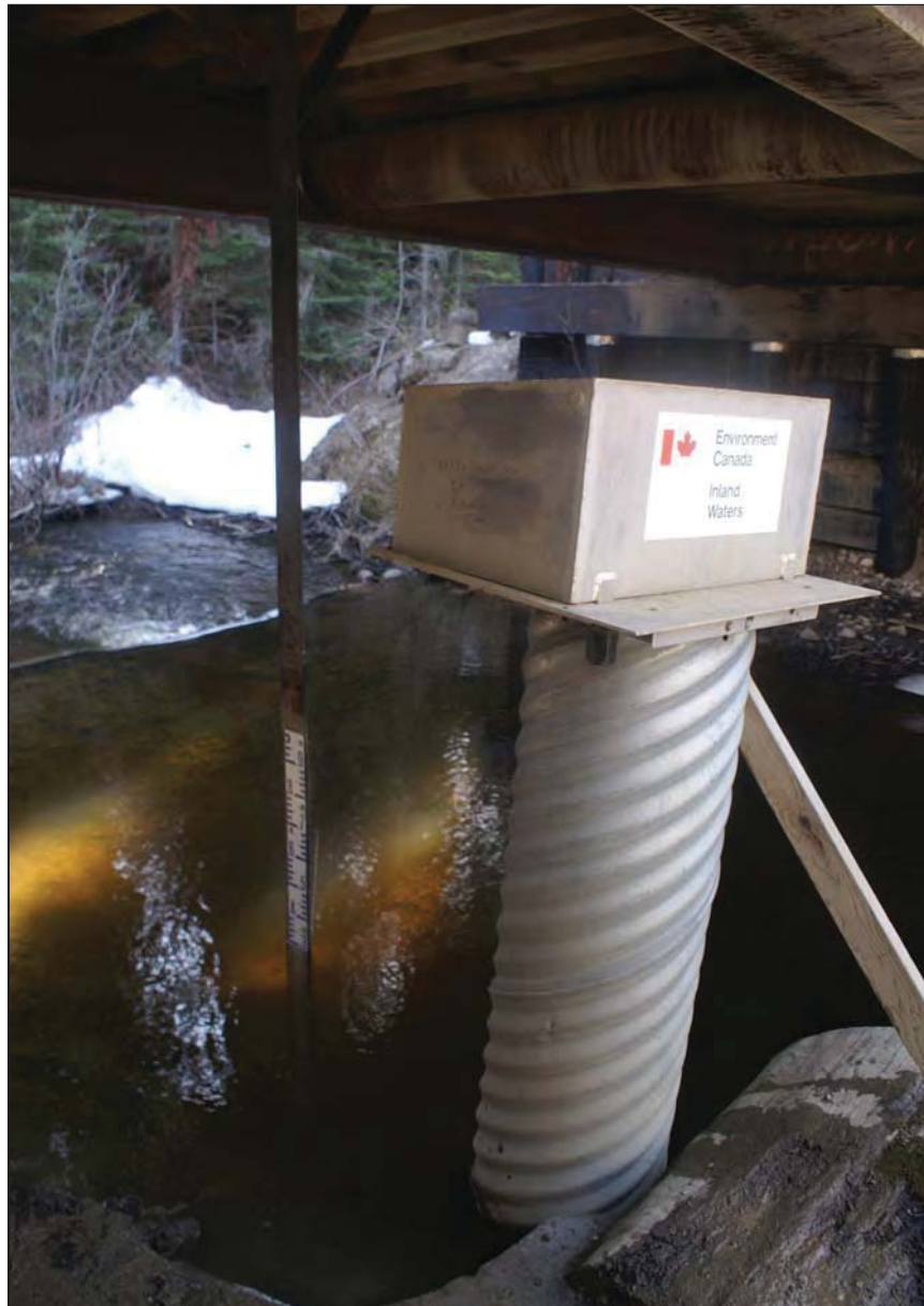
PHOTO 1 – Hazeltine Creek Gauging Station Chart Recorder and New Staff Gauge. Photo taken in April 2010 following installation of new staff gauge support. Notice that the gauge Height is ~0.300, and water level is at the weir crest.
