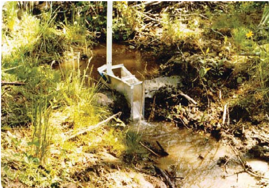
Figure C-32. Three-inch Montana flume set in temporary silt “dam”.
