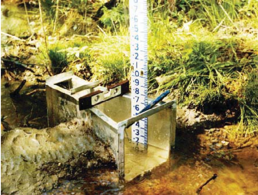
Figure B-5. Three-inch Montana flume set in a mud dam.
