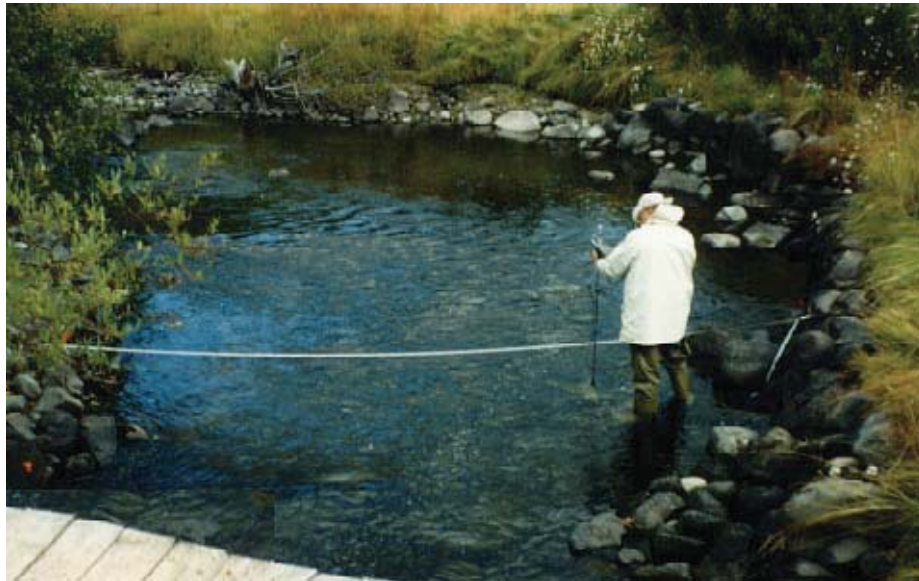
Figure D-4. Conducting a discharge measurement with tagline across the wading section, Bridge Creek below Dekka Creek.
