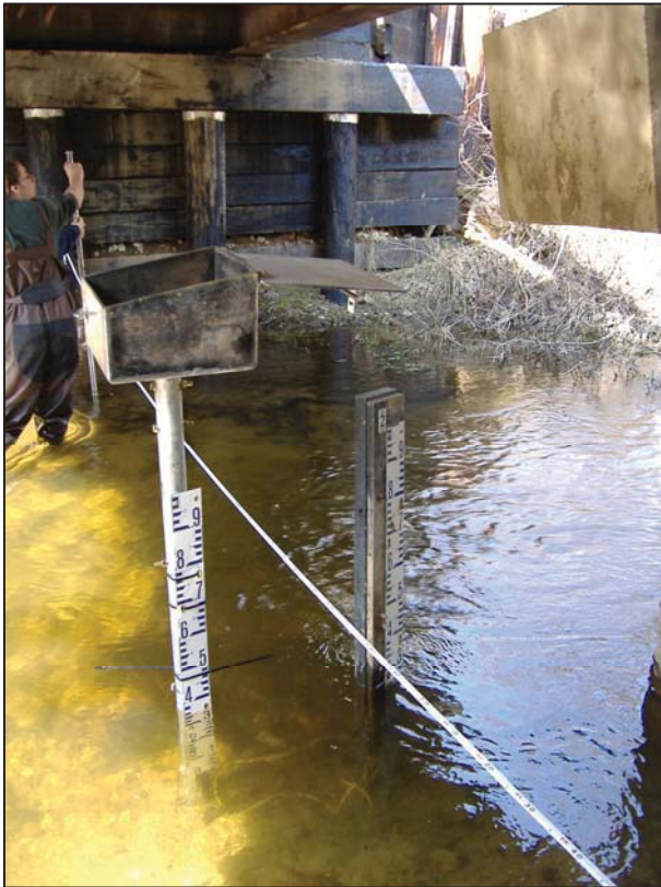
PHOTO 1 – Hazeltine Creek Gauging Station (H7). New gauge plate and datalogger installation located downstream of existing gauge plate, with 0.100 m offset between gauges.
