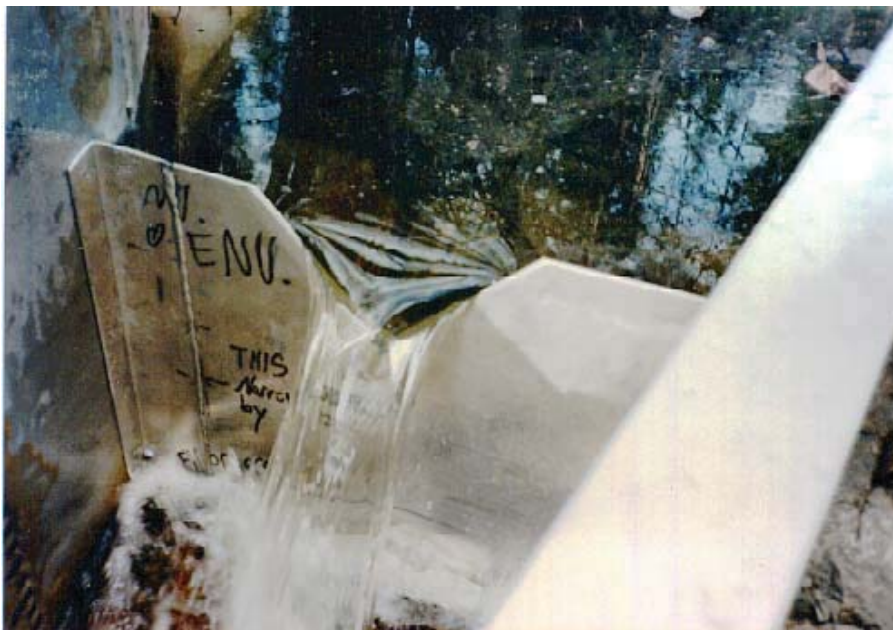
Figure C-34. Small V-notch weir plate inserted across flume entrance.
