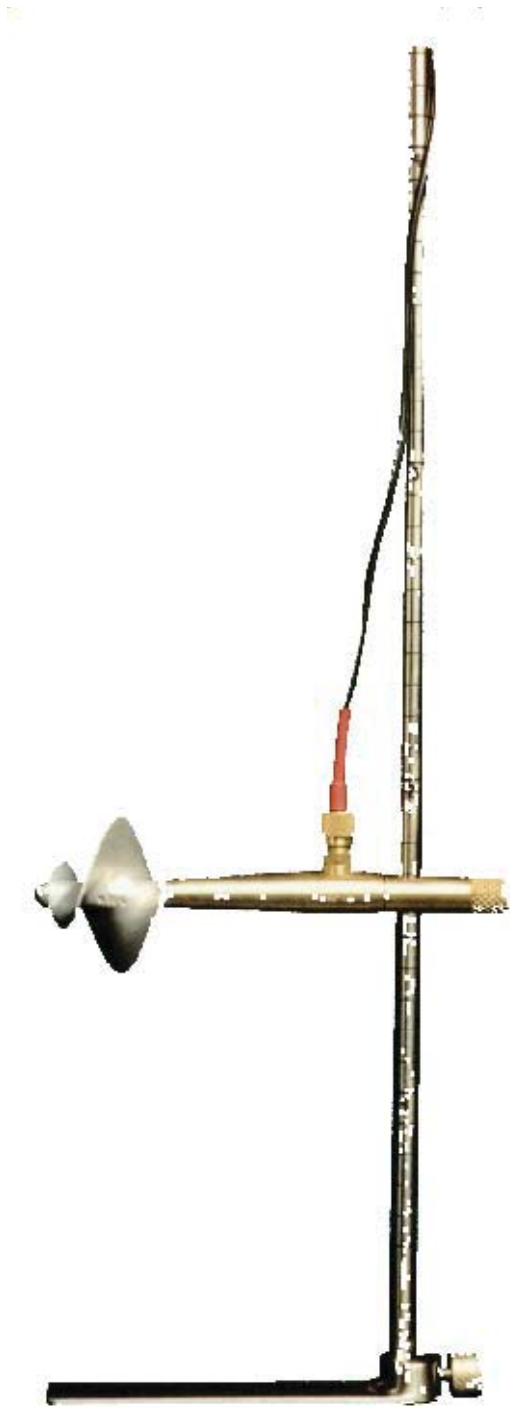
Figure C-20. OTT C2 current meter, mounted on a 9-mm rod.
