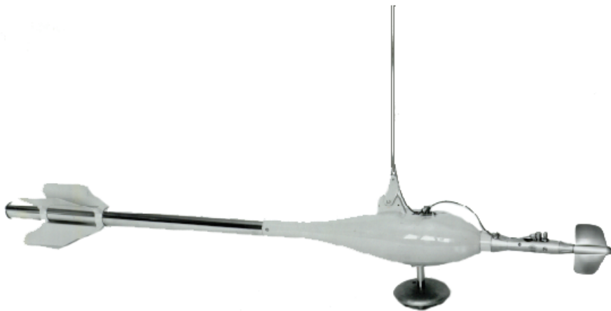
Figure C-25. OSS B1 current meter mounted on a 30-kg sounding weight (middle), with a bottom feeler.
