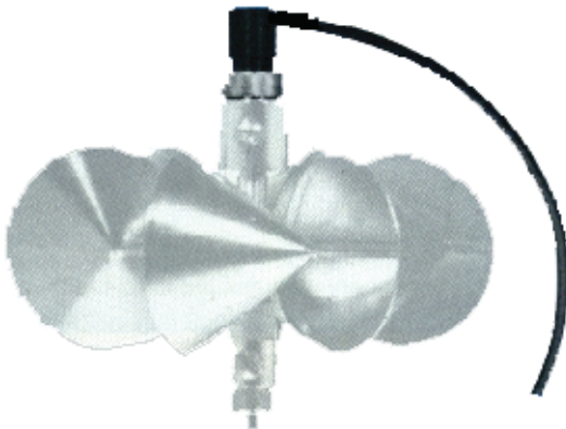
Figure C-17. Fibre optic retrofitted Price 622AA.
