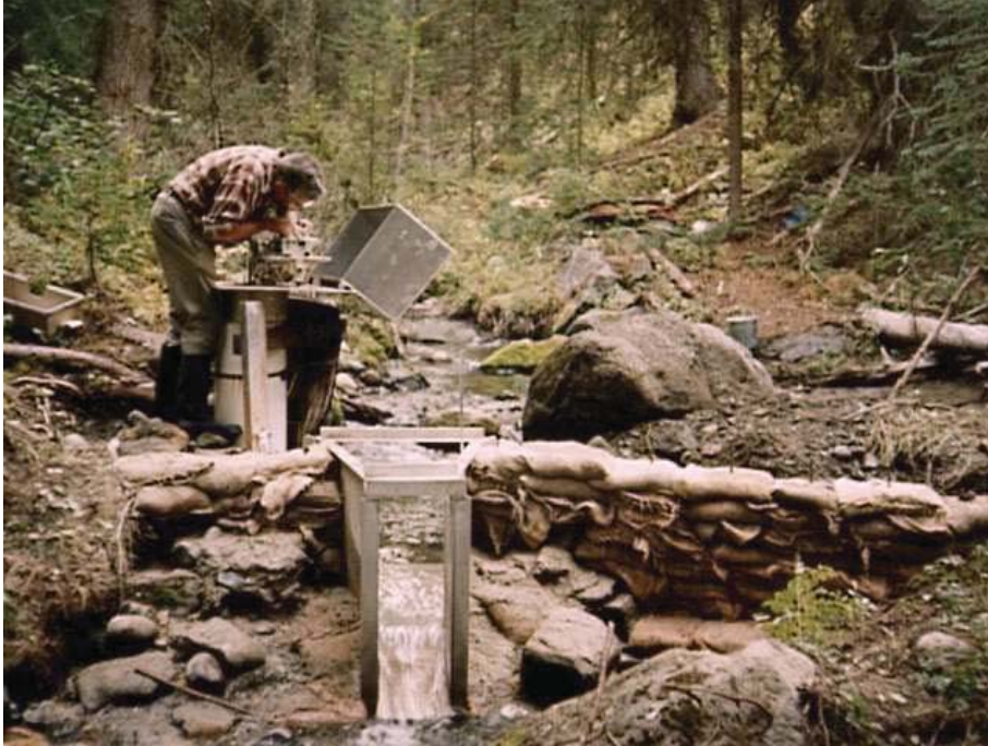
Figure G-5. 6-inch Montana Flume set in concrete sack bulkhead. Bidwell Creek above Chilko River.
