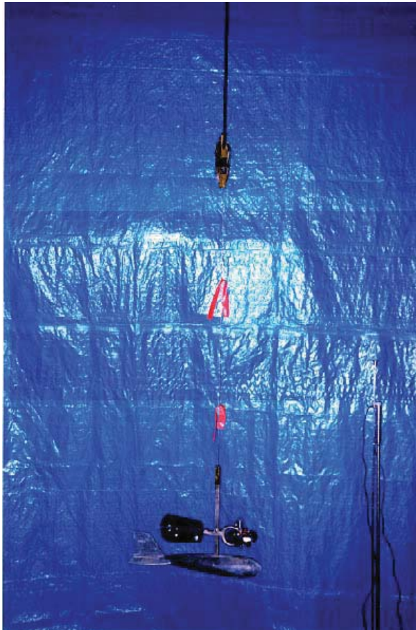
Figure D-10. Handline-suspended meter and Columbus weight. Just over 1 m of sounding cable unwound from reel. Tags 0.5 m and 1.0 m above centre of meter.
