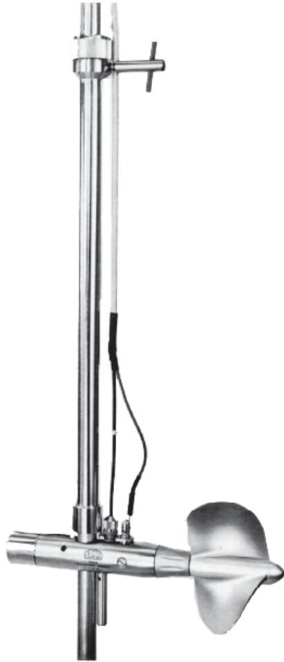
Figure C-24. OTT C31 current meter fitted on a 20-mm rod, with relocating device. Note that the locating device, at top, is aligned with a meter.
