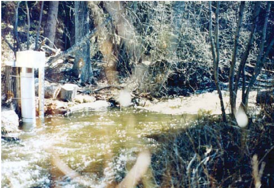
Figure B-4. Boulder control (subject to debris build-up) and water level recorder stilling well and shelter. Narcosli Creek, above Ramsay Creek, West Fraser.
