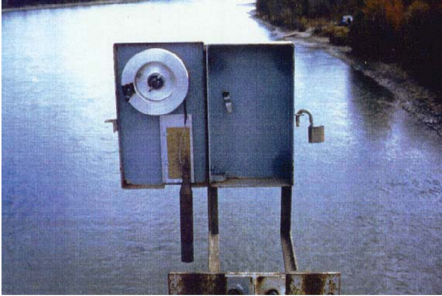
Figure B-16. Wire-weight gauge and mounting brackets. Athabasca River, near Windfall.
