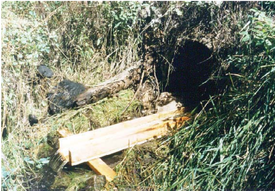
Figure B-7. Culvert with low outlet and flow led into flume for volumetric measurement.
