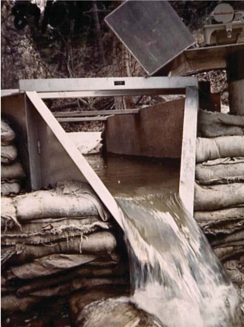
Figure G-3. 2.5 foot H Flume set in concrete filled sacks. Cuisson Creek above Gibraltar Mine.
