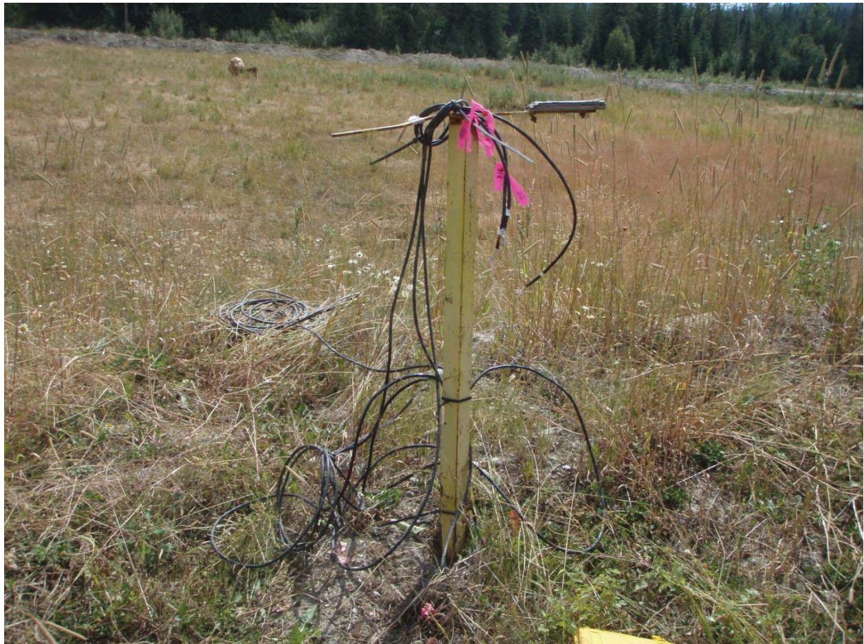
Piezometer below filter stockpile at the bottom of corner 2. B14, B15, B16. Labels put onto wires today.
