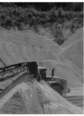
This picture is of the discharge end of the manufactured fines conveyor. No visible dust could be seen coming from neither this belt nor any other conveyor discharge that was observed during this inspection.
