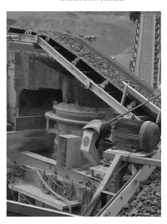
This picture is of the cone crusher for the manufactured fines. This area does produce a small amount of dust which appears to be from the crusher drive motor and belts pulling dust from the crusher. This dust was not of any quantity that would migrate from this local area but could be hazardous to unprotected workers working in this area. Once again this possible worker exposure needs to be evaluated by Valley Black Top/Selkirk Paving.
