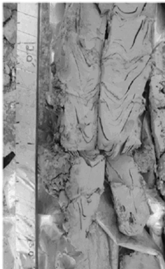
Disturbed clay below failed embankment area
