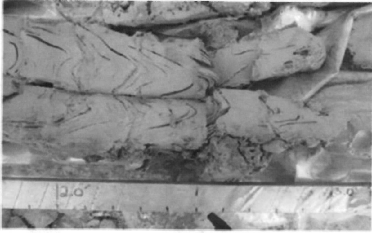
Disturbed clay below failed embankment area
