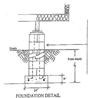
Chessis beam Shims Blocking as required
