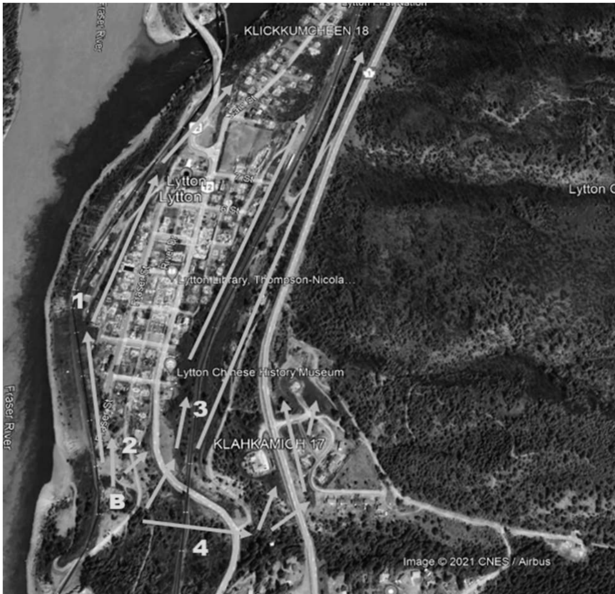
Figure 3: Arrows trace the estimated eventual Spread Paths of wildfire that exposed Lytton Village, IR 18 and IR 17 to flames and burning embers that initiated community ignitions
