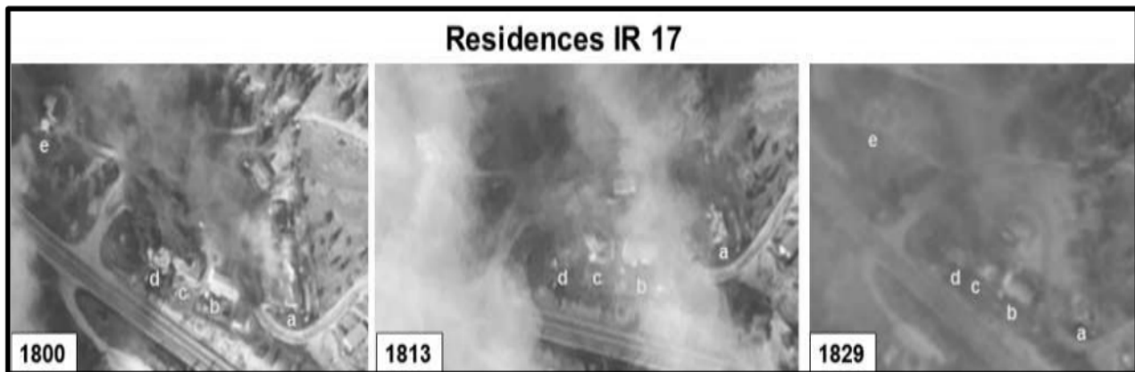
Figure 13: Time progression of 5 destroyed houses in IR 17. Each photo references the houses with yellow letters a – e.
