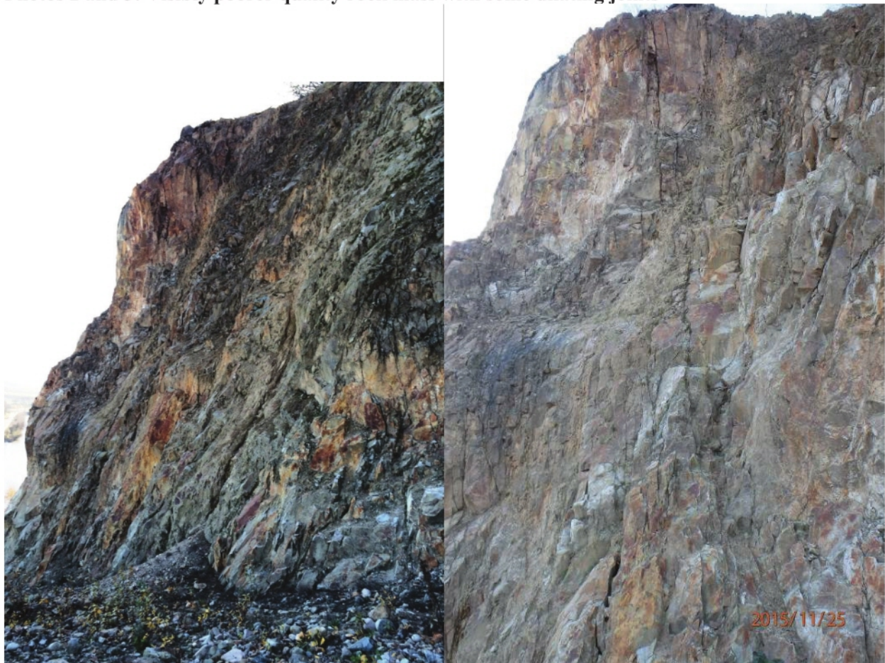
Photos 2 and 3: Visibly poorer quality rock mass with some dilating joints
