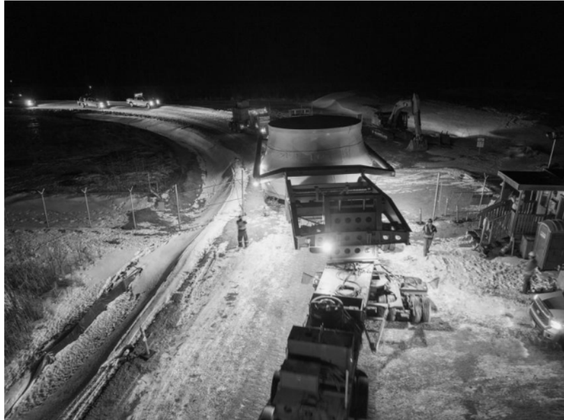
Figure A-3 Unit 1 turbine runner arrives at Site C after travelling from Sao Paulo, Brazil, by ship to Prince Rupert, and transported on a customized truck to the project site (January 2021)
