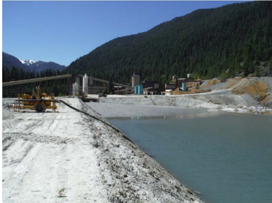
Figure 17. A pump used to remove supernatant water from the surface of the tailings.
