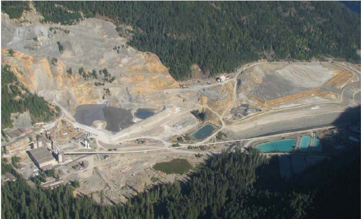
Figure ES-1. Aerial view of the Myra Falls mine showing the Lynx TDF on the left. The darker gray surface is the top of the tailings; the light gray to the right of the tailings is the embankment dam of rockfill; the brown and gray mottled areas to the upper left of the tailings are the steep slopes of bedrock and the waste rock piles above the Lynx TDF. (From AMEC 2013a)
