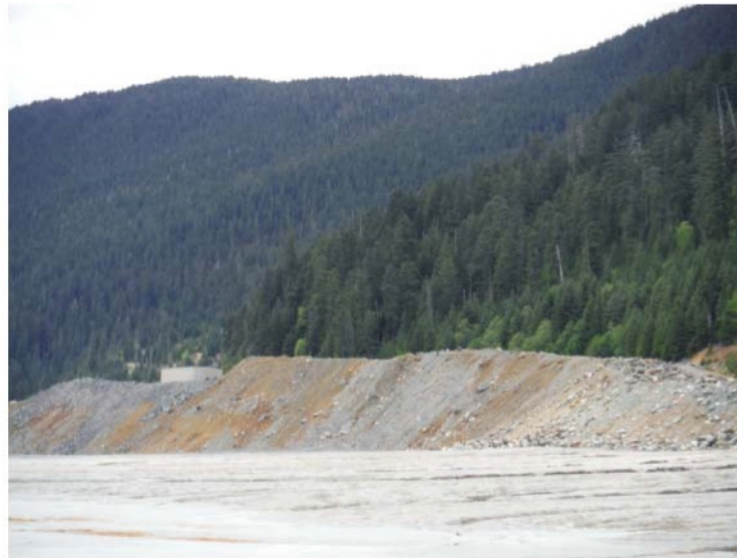
Figure 5. The south face of the waste rock dumps rising from the surface of the paste tailings area.
