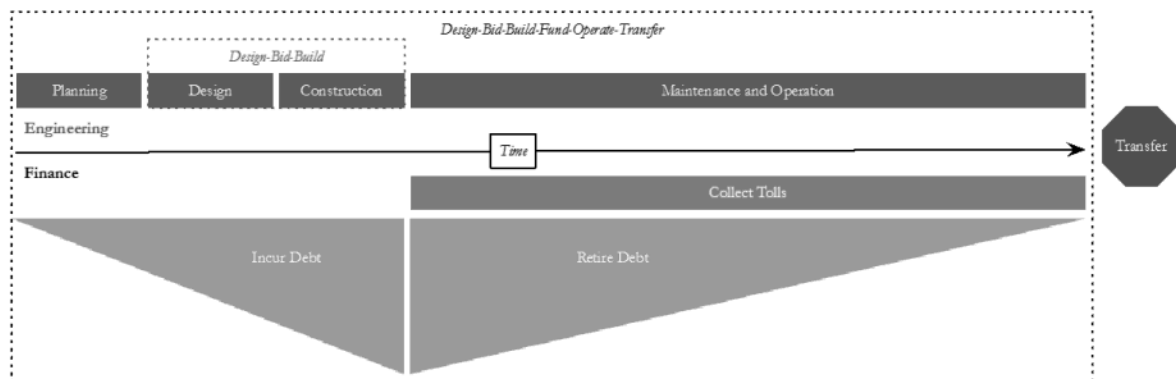
Figure 9: Principal Elements of a Tolled Highway Project
