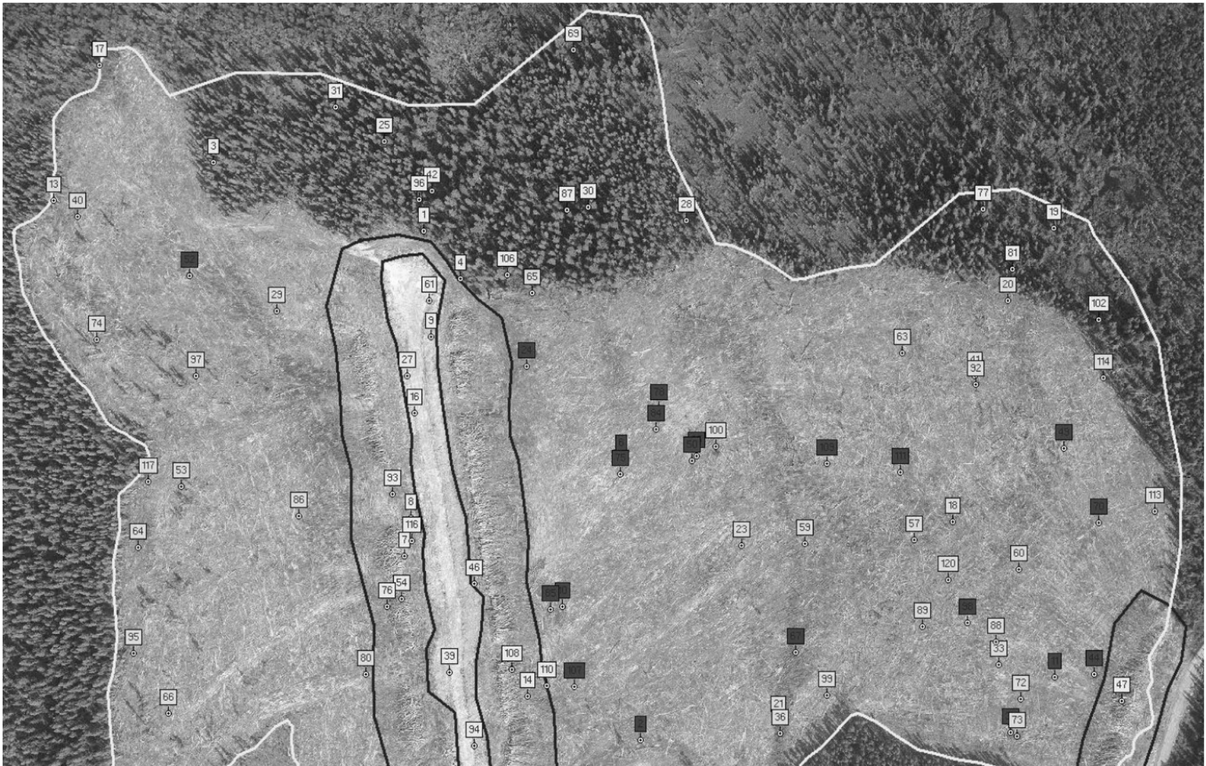
Figure 2. GPS soil survey map (north end): Waypoints are identified as non-counted disturbance ( yellow ), counted disturbance ( red ) or point landing outside of NAR ( grey ).
