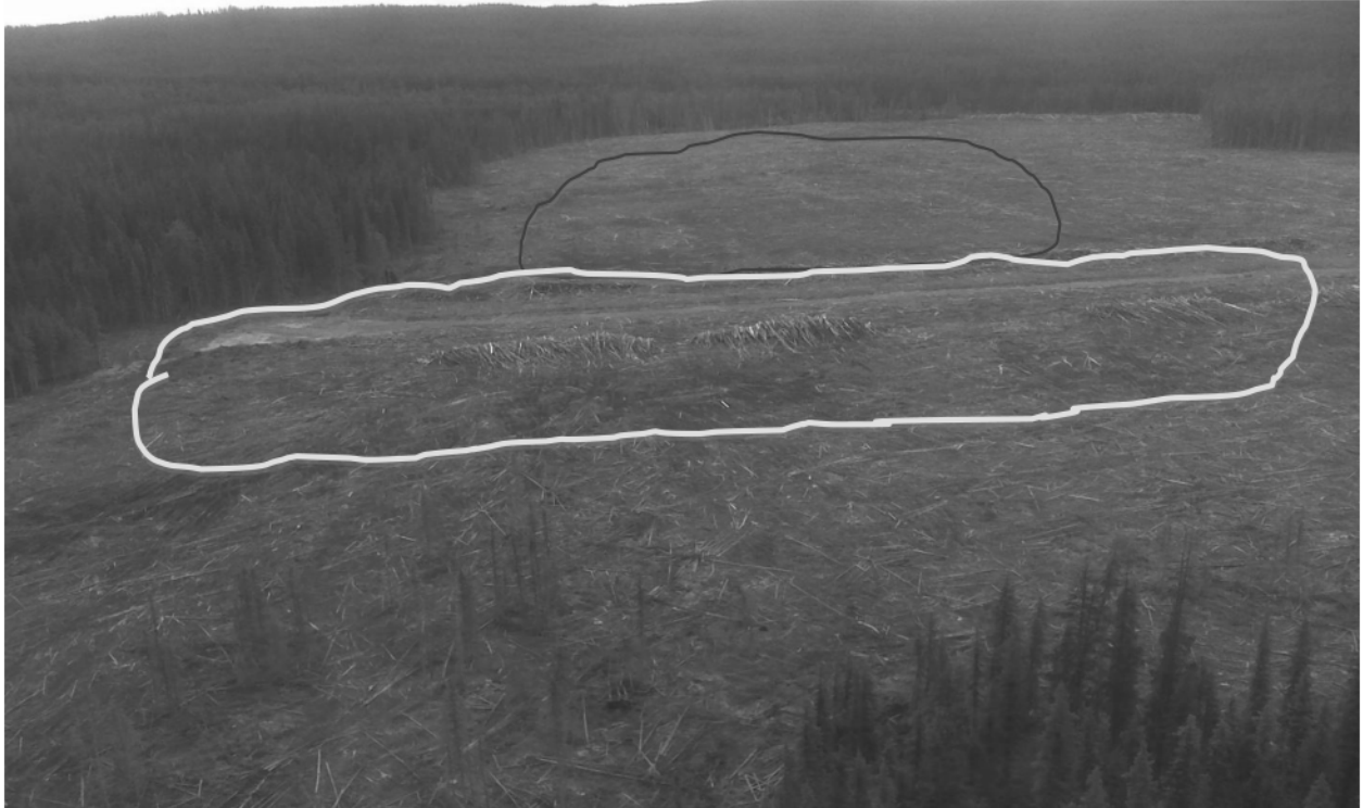
Looking northeast, large compacted area >1 ha (red perimeter) and RWA disturbances
