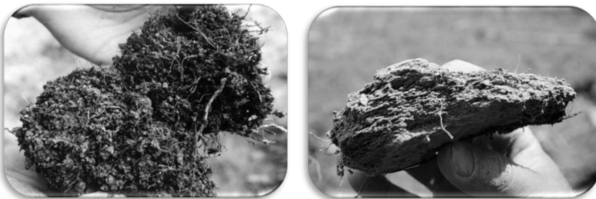
Figure 5. Example of the compaction process: Fluffy or loosely arranged soil (left) turns into compacted structure (right) during logging when soil is wet. Water flow and nutrient uptake by plants are impeded therefore can decrease site productivity.
