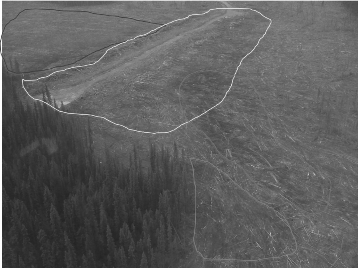
Looking northeast, same compacted area >1 ha, RWA disturbance and area of concentrated disturbance (orange perimeter) and impeded drainage (blue perimeter).
