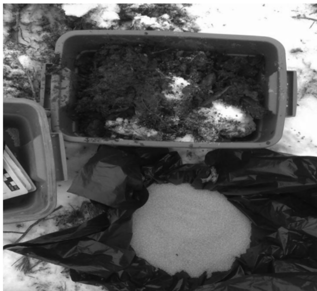
Bulk density sampling by excavation
