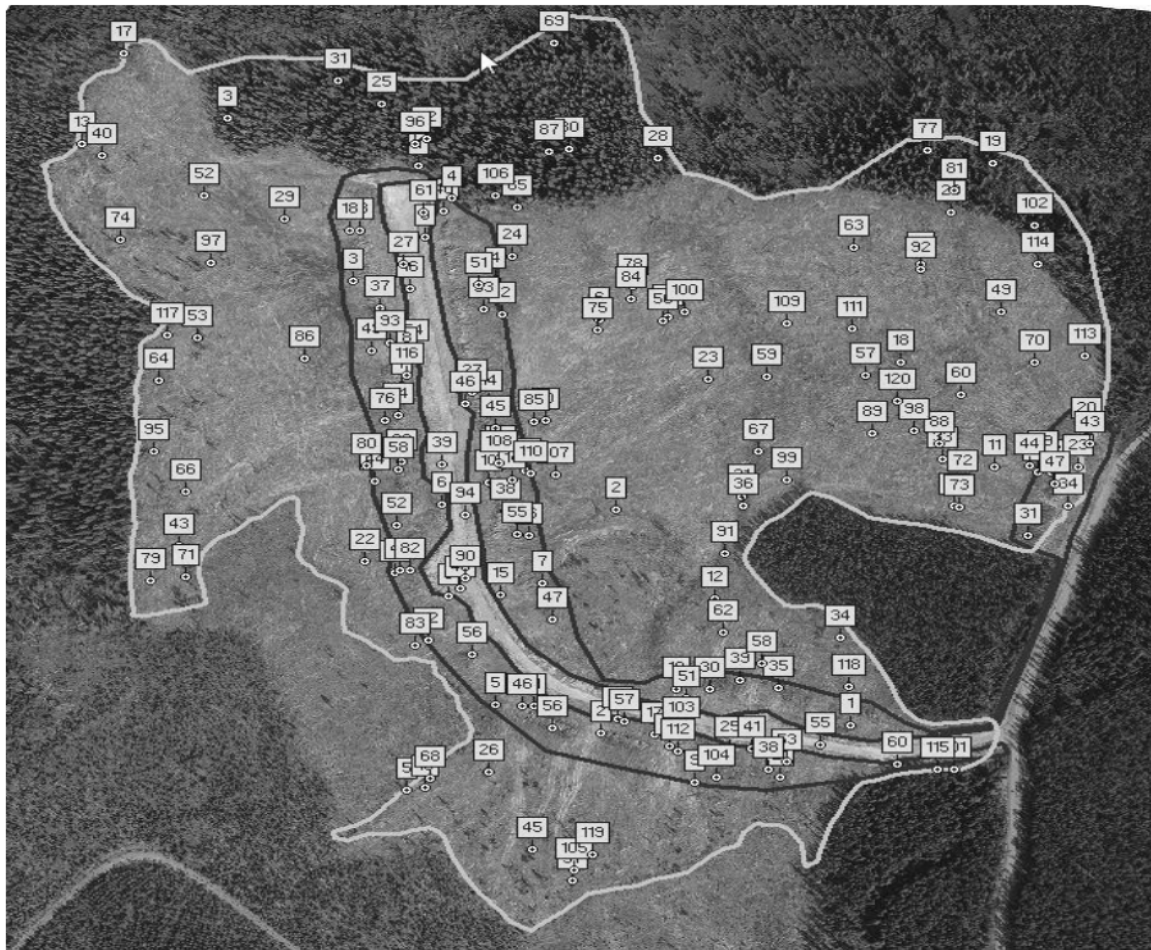
Figure 1. Aerial Photography of block A72921 CP008 CB18 taken in 2012 (1 year post logging, 15 cm pixel size resolution). GPS soil survey map showing random sampling points (or GPS waypoints with Latitude and Longitude coordinates) with yellow symbol in NAR (grey perimeter) and RWA's (blue perimeter).
