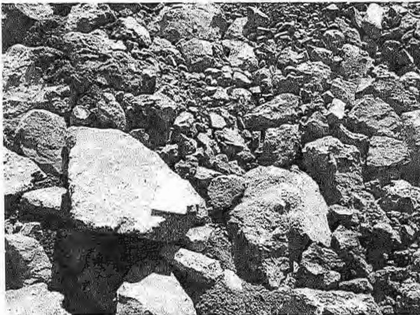
FIGURE 2: ROCK CRUSHED BY DOZER
