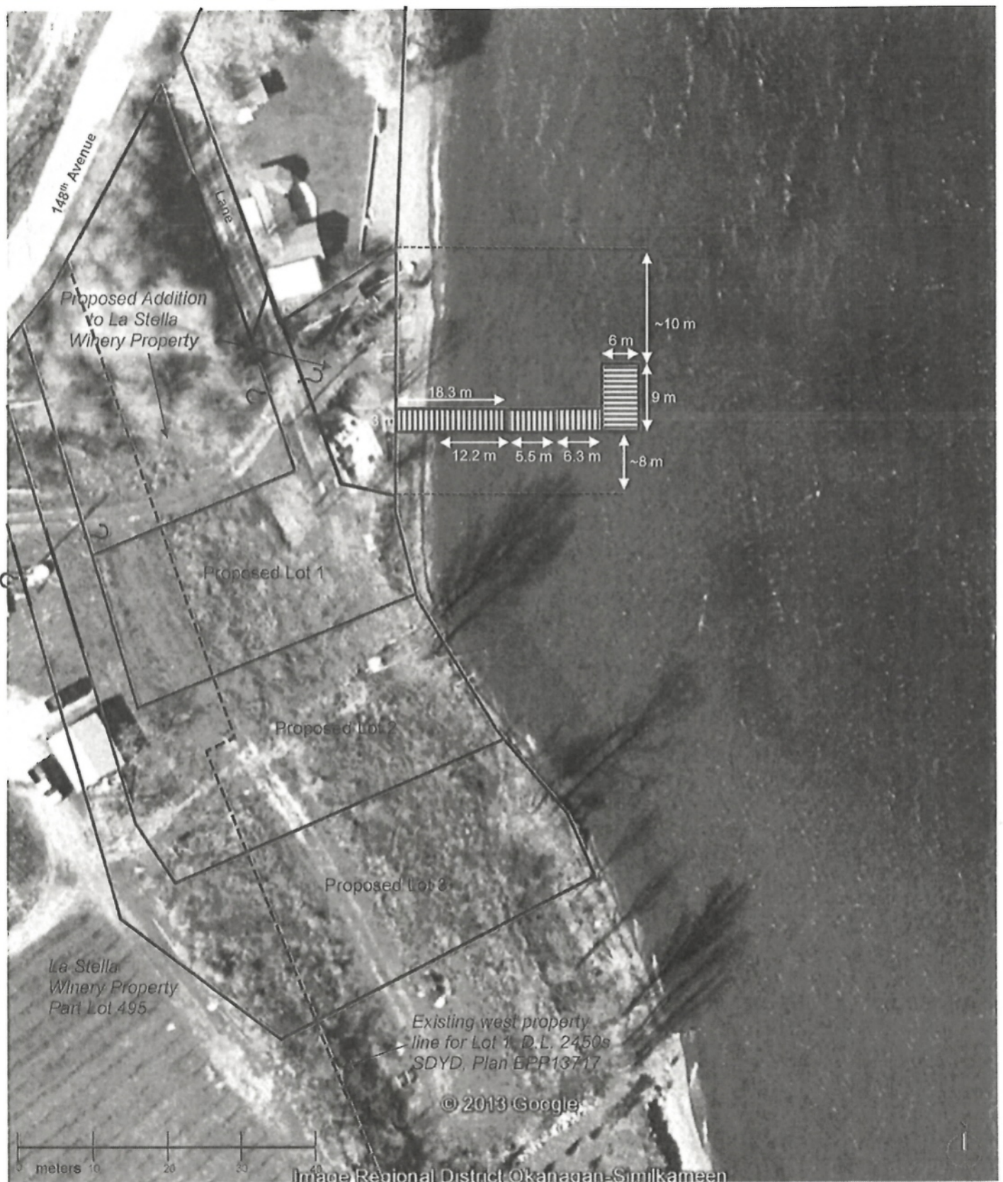
Illustration 3: Proposed Dock Dimensions and Details – Plan View
