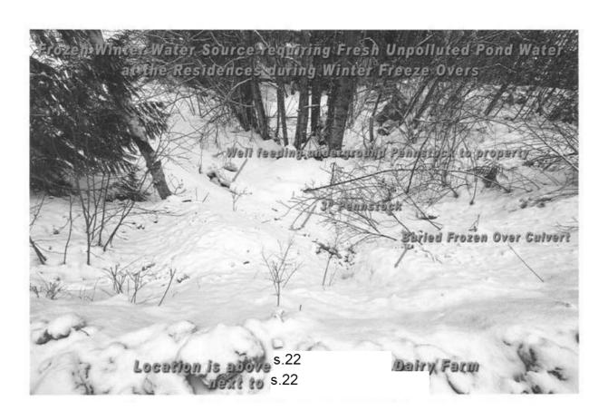
The attached pdf was created Feb 2, 2014. The Penstock is in fact buried 4' underground for one kilometer down to the house and winter drinking pond. It's the "water intake culvert" above the polluted farm a kilometer South which totally freezes up and that's the problem. Without the winter drinking pond, how am I going to get my 1000/gallons per day of domestic water in January and February as has been done since day one?
