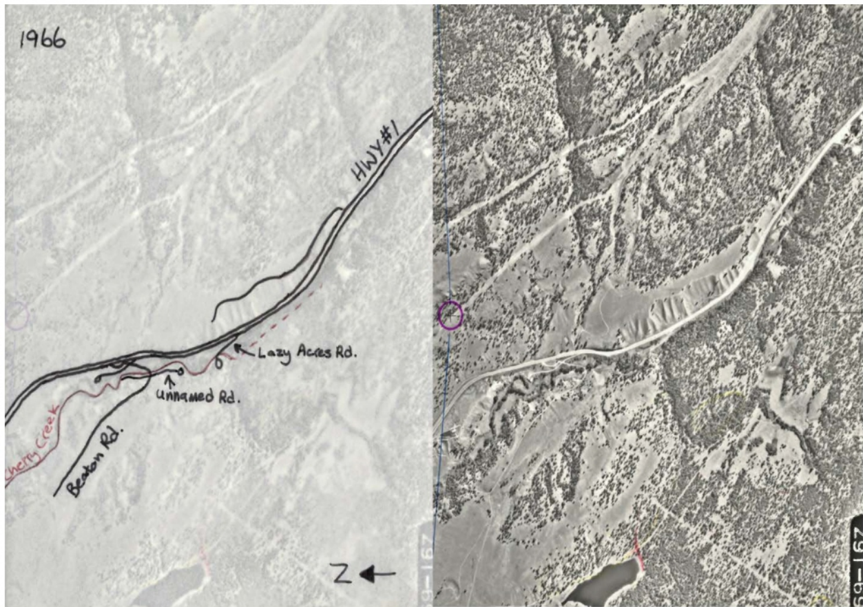
Figure 2. 1966 Air Photo Composition. The image on the left shows an overlay with road and creek interpretation, the image on the right shows the original imagery.
