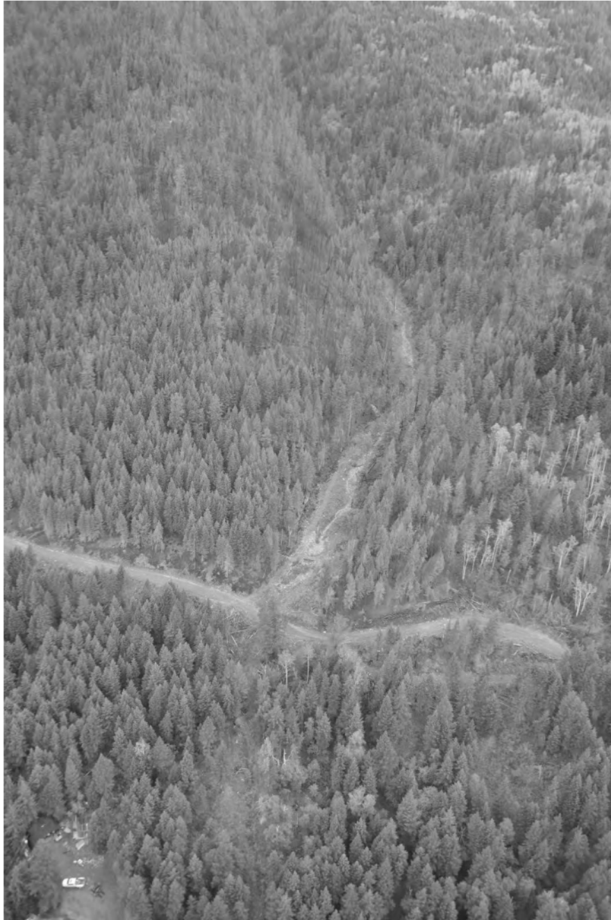
Plate 5: Looking upslope along watershed WS2. The debris flood from 2017 cleared trees along the margins of the draw making the channel wider. The trace of the creek can be seen at lower centre.
