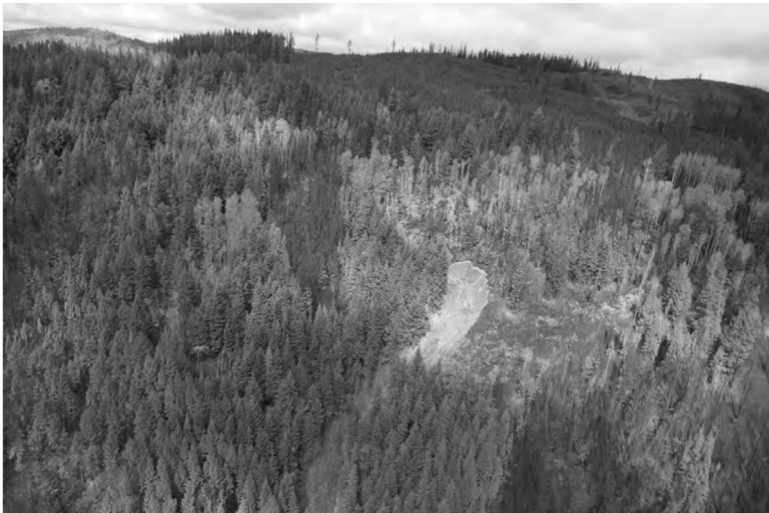
Plate 4: Headscarp of the 2017 landslide (debris flood) which ran out through watershed WS2. The upper plateau surface is quite gentle, moderately burned and was harvested between 2001 and 2017.
