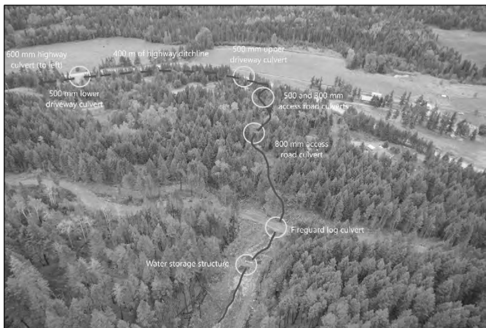
Photo 5: View looking south of the WS2 Creek alluvial fan above the HLCR. The creek passes through a number of culverts and then follows the highway ditch-line to the east before draining south into Christian Creek.
