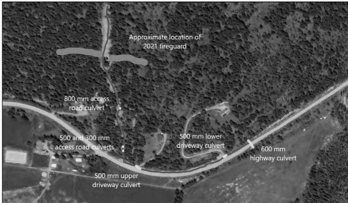
Figure 5: Google Earth view of the WS2 Creek alluvial fan from 2017. The track of the debris flow can be clearly seen coming off the upper slopes, running through the residential area, before reaching the HLCR. The creek currently follows the highway ditch-line east for 400 m to a 600 mm culvert, which passes it into the field below and then into Christian Creek.
