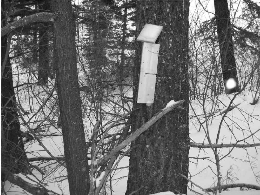
Photograph 1. Hair detector attached to a tree with roof above and run pole beneath.
