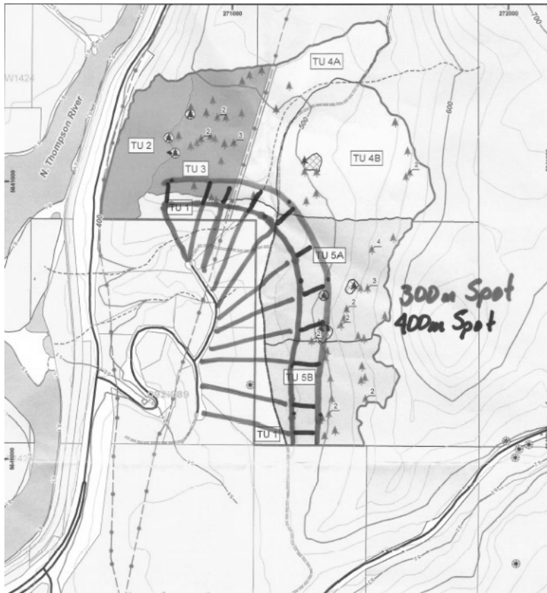
Figure 8. An ember/spotting impact map showing the depth into the treatment units where a spotting ember could impact the community (red area is 300 meters from the community, the black is 400 meters from the community).
