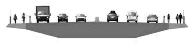
Potential future conversion to a six-lane bridge; multi-use paths could be added on either side of the bridge for pedestrians and cyclists.
