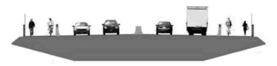
Four-lane bridge with two-way pedestrian and cyclist facilities separated from traffic on both sides of the bridge.
