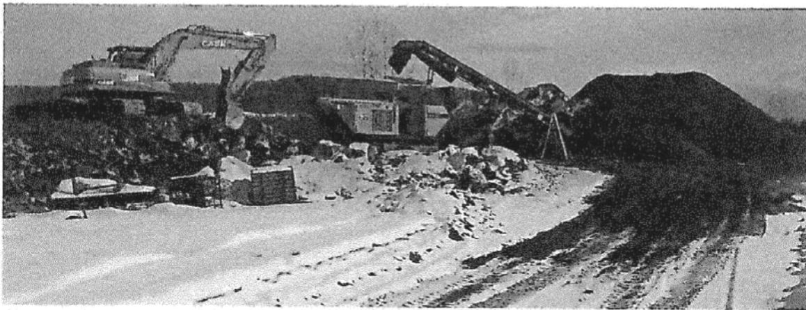
Above: waste concrete reprocessing produced 5600 m 3 of aggregate suitable for road bed construction, driveways, parking lots. Below: Equipment and shop facilities at Mounce property.
