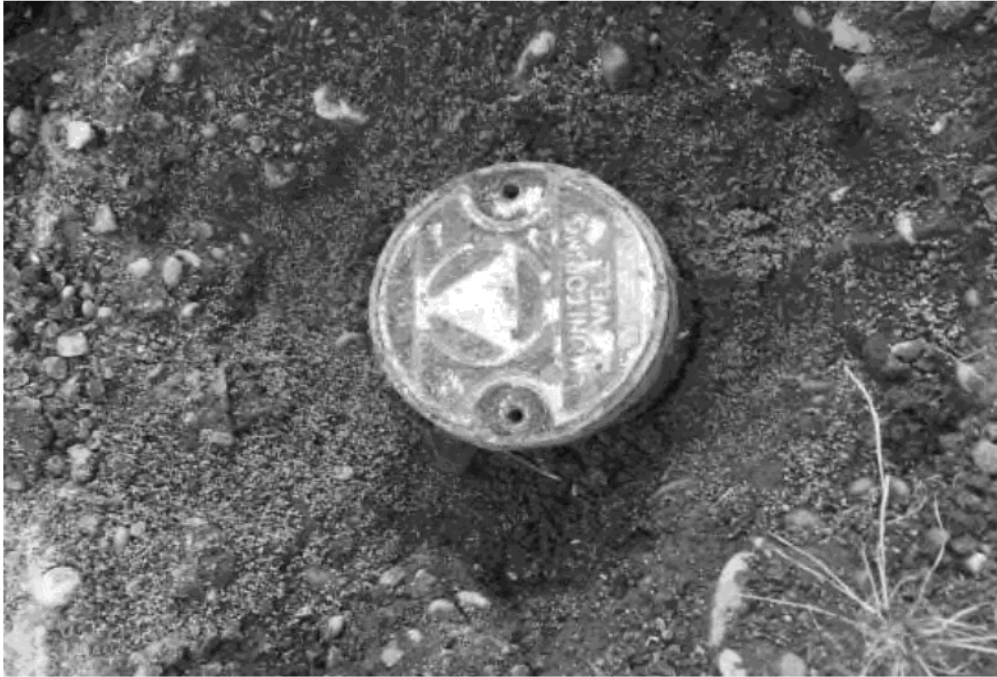
Photograph 5: Viewing the exposed metal casing at the ground level of the monitoring well MW15-9.
