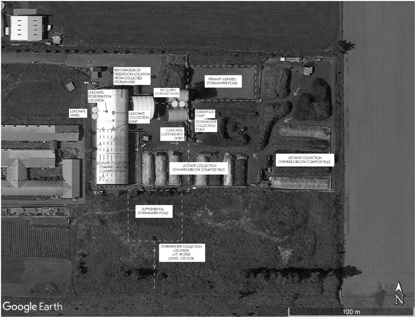
FIGURE 4. STORMWATER AND LEACHATE MANAGEMENT SYSTEMS
