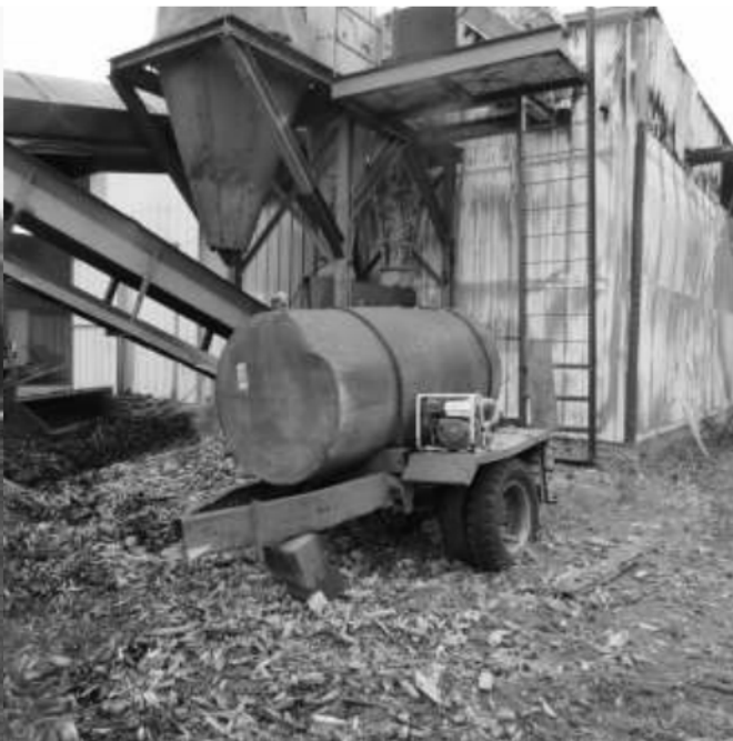
Photo #8 Water tank empty over the winter. Mill not sprinklered - No FD water supply.
