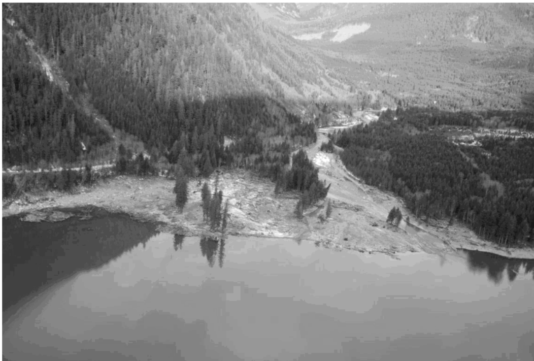
Photo 12: Aerial view of damage caused to the campground at the north end of Chehalis Lake. The wave run-up measured on the shoreline at the far left of the above photo was 23 m.
