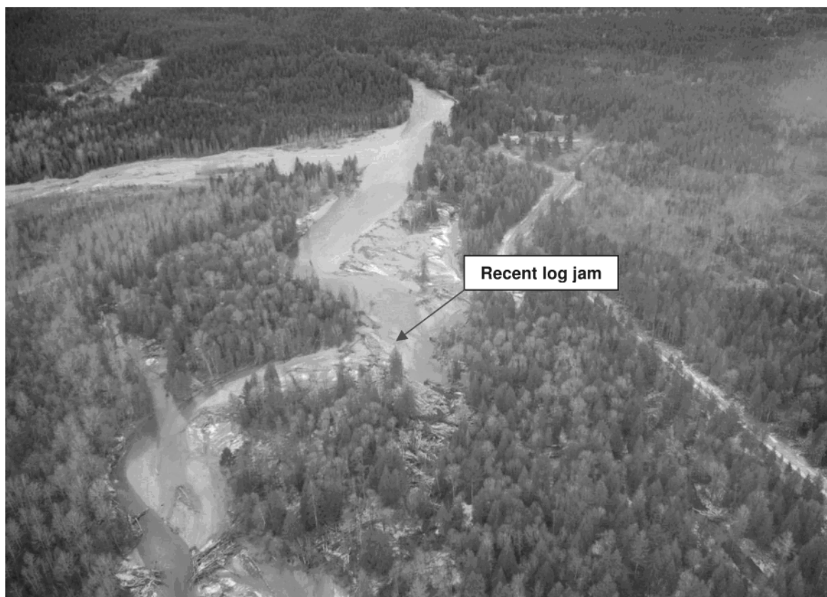
Photo 17: Upstream view of Chehalis River on the alluvial fan. The recently constructed dyke is visible on the right side and an arrow points to a log jam that is likely associated with the rock slide and/or recent storm.
