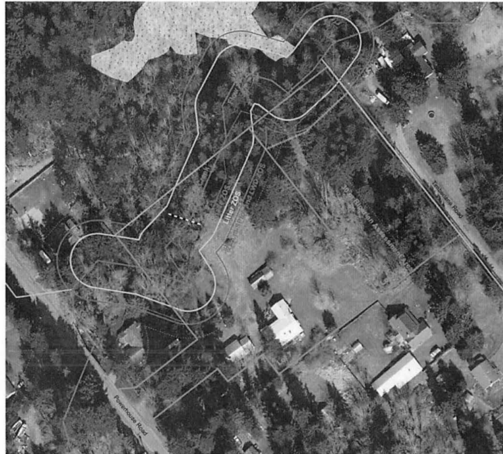
Figure 1. Site plan of subject property from Riparian Areas Regulation assessment showing calculated SPEA setbacks for Morrison Creek (red line) and the ditch along Timberlane Road (Purple line).
