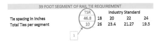
1. In the application of the minimum requirement for Class 3 Track under the TSR tie spacing would be 46.8 Inches (39 foot segment of track X 12 Inches = 468 Inches / 10 ties = 46.8 Inch tie spacing.)
