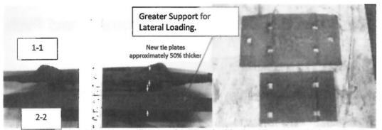
Do note that in the above photos illustrated 1-1 is a double shoulder plate which is normally thinner than a single shoulder. Additionally both photos illustrate a 5 ½ inch base used for 100lb rail. Rather than the 5 3/16 for 85lb rail presently in place at the VIRC. As per below this reinforces the importance of not only better tie plates but rail upgrades to at least 100lb. in key locations.
