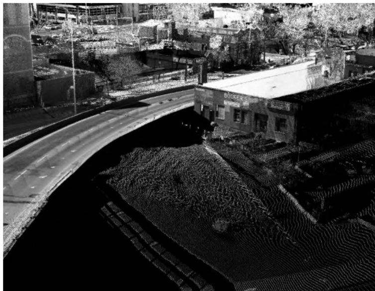
LiDAR Point Cloud Colorized Using PSP Digital Images
