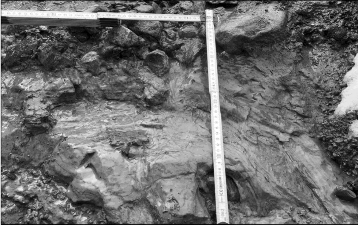
PHOTO 5: View of silt layer exposed in landslide track.
