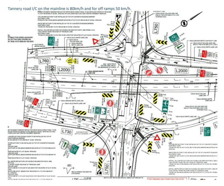
Hwy 99 I/C on the mainline is 80km/hand on off ramp 50 km/h.
