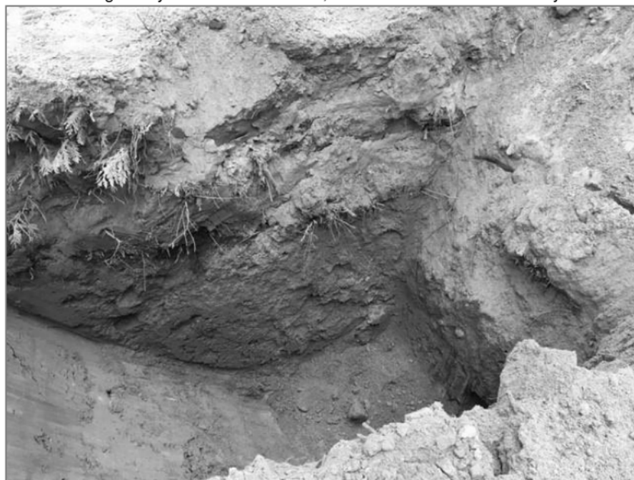
Photo 2: Testpit conducted at the toe of slope. Intermediate topsoil horizons indicating historic layering of colluvial deposits. Loose sand encountered through to end of testpit at a termination depth of 3.5 m.
