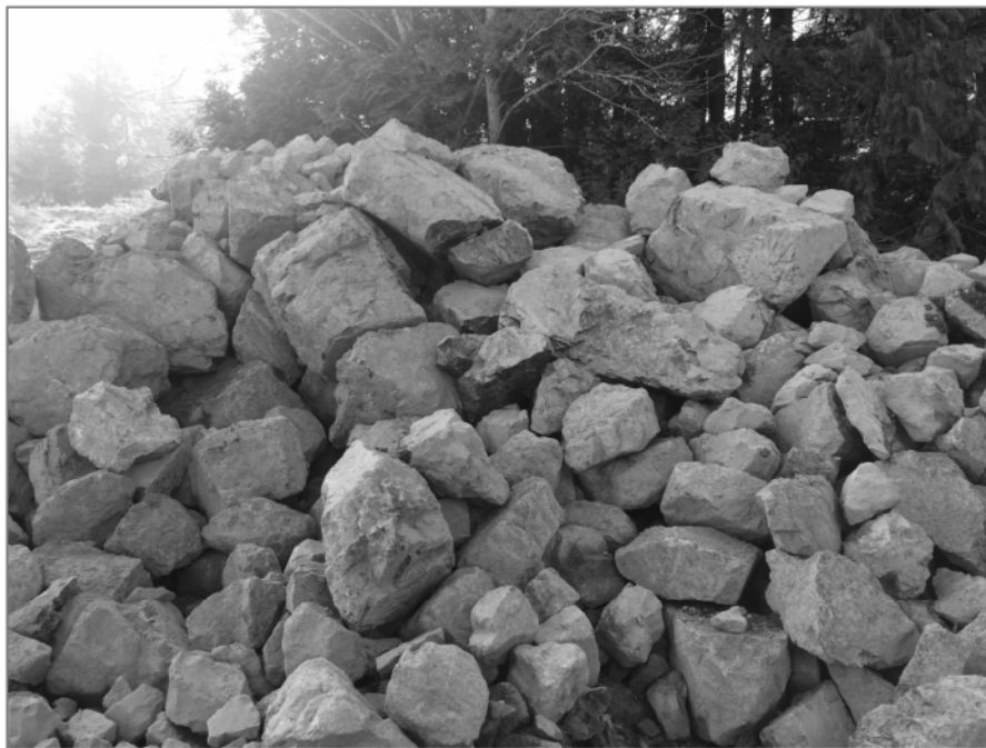
Photo 2: Photo of angular riprap inspected and approved prior to use.
