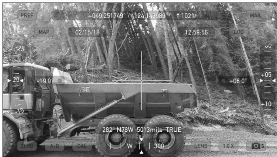
Photo 5: Slope inclinometer image indicating the access ramp is approximately 20 degrees.
