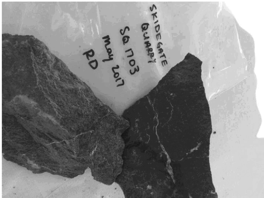
SQ1703 Description: green-grey andesite with trace sulphides, red hematite is present throughout matrix. Calcite vein is present throughout the sample.
