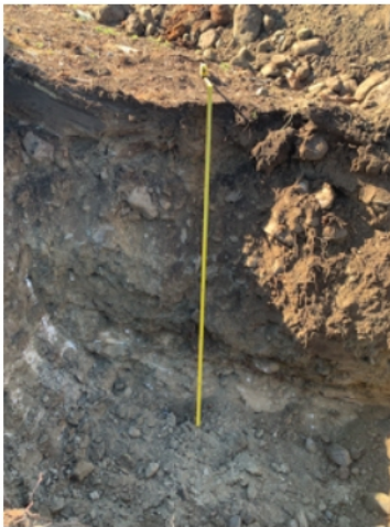
Photo 9: Test pit, typical morainal outwash soil over bedrock at 640m elev, SW corner of property
